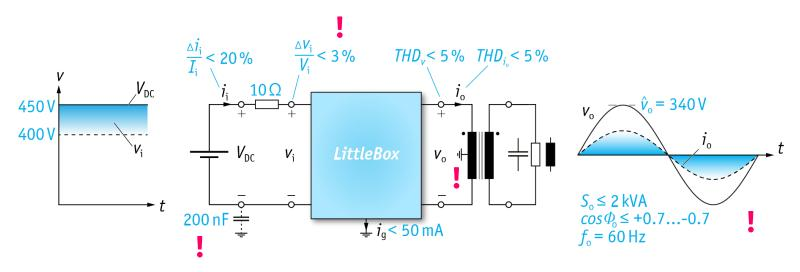
Push the Forefront of New Technologies in R&D of High Power Density Inverters
