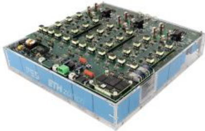
★ 7-Level All-Si HANPC PV Inverter 99.35% @ 3.4 kW/dm 3
