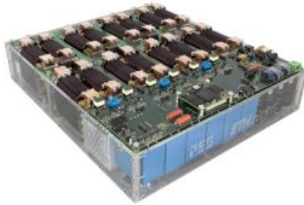
★ 3-Level All-SiC T-Type PV Inverter 99.4% @ 2.4 kW/dm 3
