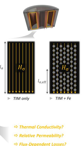
**Thermally Conductive Epoxy Resin** to be mixed with magnetically conductive powder (iron or ferrite particles)
