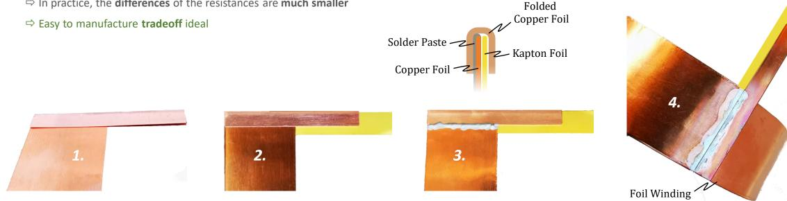
Winding Terminal Manufacturing Sequence: 1. folding the copper foil around the end of the winding, 2. slide Kapton foil into folded copper foil, 3. add solder paste on the top side copper interface, 4. solder copper interface
