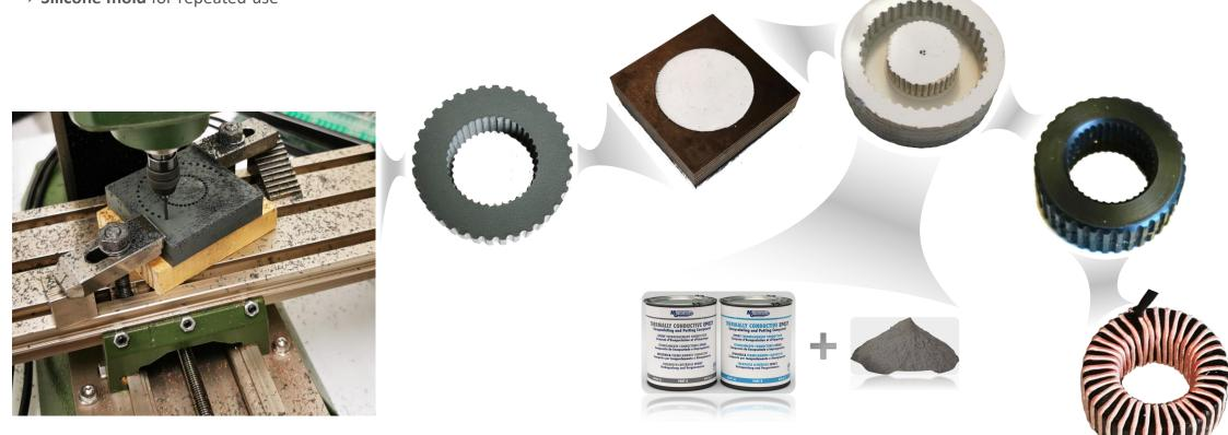
Manufacturing Sequence of the silicone molds used as the negative form of the final inductor cores
