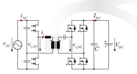
Bidirectional Isolated AC/DC Converter (Buck/Boost)
