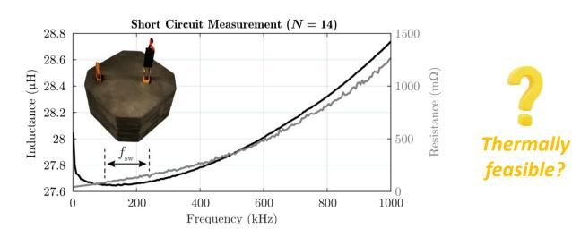
Impedance Analyzer Measurements of the transformer with a shorted secondary side winding
