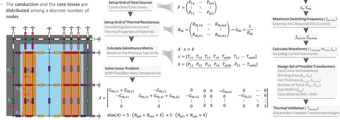
**Thermal Model** for estimating the temperatures in foil winding transformers for certain given conduction and core losses
