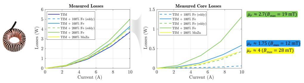
Loss Comparison of different core materials at 110 kHz for different inductor currents and flux densities – dashed lines = resistive losses (impedance analyzer) / solid lines = total losses (calorimetric measurement)
