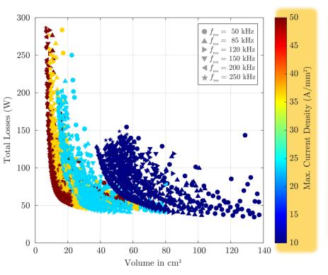
Optimization Results of foil winding transformers for the specifications of the application at hand
