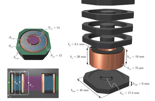
**Transformer Dimensions** and winding arrangement of the foil winding transformer
