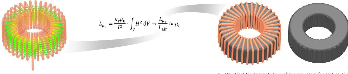
FEM Simulation Result of a toroidal inductor arrangement suitable for the measurement of the relative permeability and the core losses of a material Practical Implementation of the inductors for testing the different material properties
