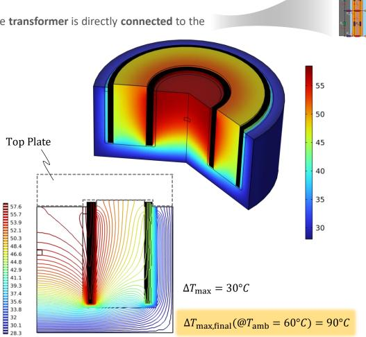
Thermal Simulation for 40 W conduction losses and a constant surface temperature of 28 °C on all outer surfaces of the transformer core
