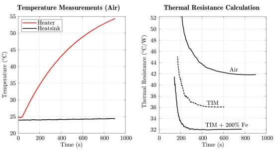
Measurement results of the different material samples by fitting the measured temperatures to a R<sub>th</sub> / C<sub>th</sub> fit-function
