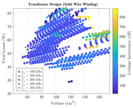
Maximum Leakage Inductance in solid wire winding transformers for different switching frequencies
