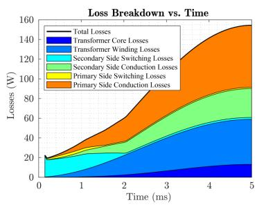
Loss Breakdown over a quarter mains period for an input voltage of 230V<sub>rms</sub>, output voltage of 470V and output power of 3.7kW
