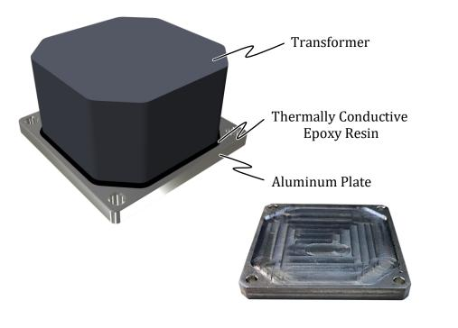
Simplified Heat Sink Design using an aluminum plate only
