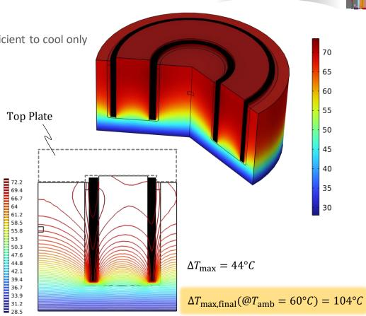
Thermal Simulation for 40 W conduction losses and a constant surface temperature of 28 °C on the bottom surface of the transformer core
