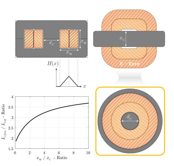
Ratio of the Leakage Inductances in a transformer with a pot core or an E-core for different winding window to core area ratios
