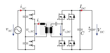
Bidirectional Isolated AC/DC Converter (Buck/Boost)
