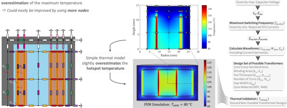
**Thermal Model** for estimating the temperatures in foil winding transformers for certain given conduction and core losses
