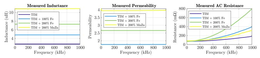
**Impedance Analyzer Measurement Results** of the different inductors/materials under test for frequencies up to 1MHz
