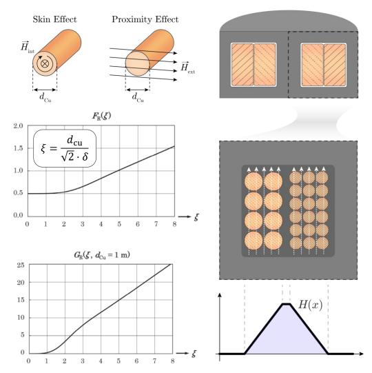
Parasitic High-Frequency Effects in different wire types due to parasitic HF magnetic fields
