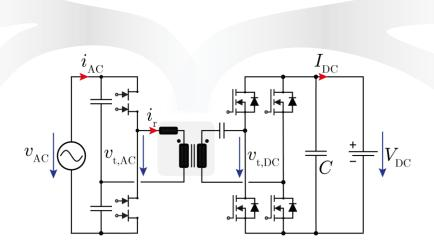
Bidirectional Isolated AC/DC Converter (Buck/Boost)
