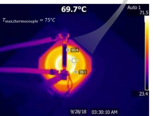
Measurement Results for hot spot temperature measurements with 40 W impressed conduction losses and a heatsink temperature of 28 °C
