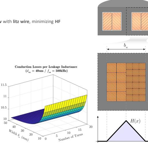
**Conduction Losses per Leakage Inductance** in a pot core transformer with litz wire (40um) windings for different geometrical parameters
