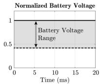
Output DC Voltage that needs to be adjusted to the momentary state-of-chargedependent battery voltage
