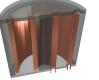
$$L_{\sigma,\text{foil}} = \frac{\mu_0 N_p^2}{3h_w} \cdot \left( l_{w,p} d_{w,p} + \frac{3l_{w,\text{gap}} d_{w,\text{gap}}}{3h_w} + l_{w,s} d_{w,s} \right)$$
