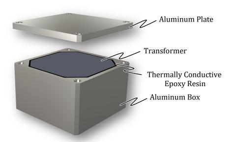
Heat Sink Design of achieving minimal hot spot temperatures
