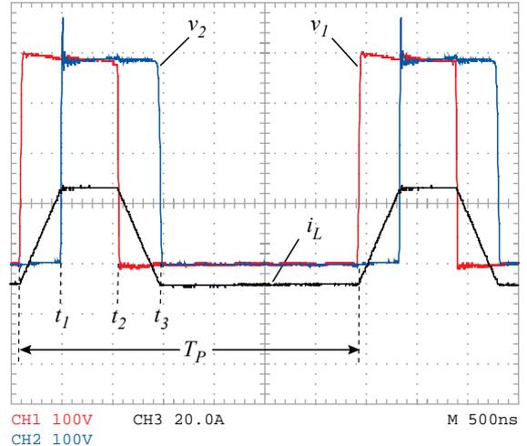
Fig. 12: Waveforms for equal input and output voltage  $V_1 = V_2 = 200$ V supplying a resistive load at 1.5 kW.
