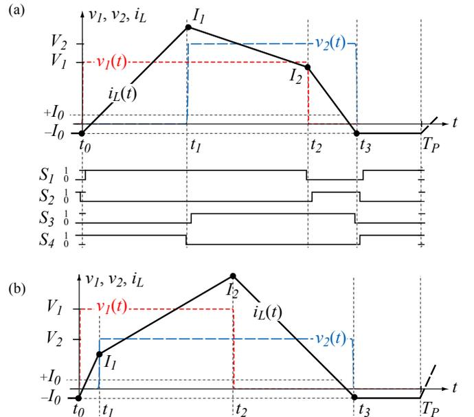
Fig. 2: Basic timing diagram for switch  $S_1$  to  $S_4$  control signals and inductor current  $i_L$  for boost operation ( $V_2 > V_1$ ) (a) and basic timing diagram for buck operation ( $V_2 < V_1$ ) (b).
