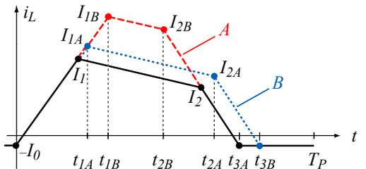
Fig. 5: Possibilities to increase transferred power  $P_{tr}$ : Keeping  $t_3$  constant (waveform A) and shifting  $t_3$  towards the end of the switching period  $T_p$  (waveform B).
