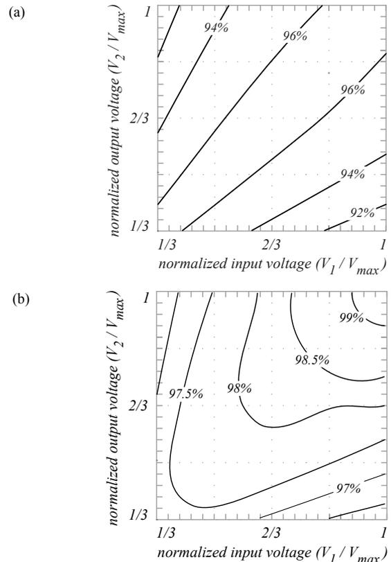
Fig. 7: Calculated semiconductor efficiency for cascaded buck+boost converter in hard-switched operation (a) and operated with the novel low-loss modulation strategy (b).
