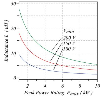
Fig. 4: Maximum inductance  $L$ , shown for  $V_{1,min} = V_{2,min} = V_{min}$ ,  $I_0 = 10A$ , and  $f_s = 100kHz$  as function of the converter peak power rating  $P_{max}$ .
