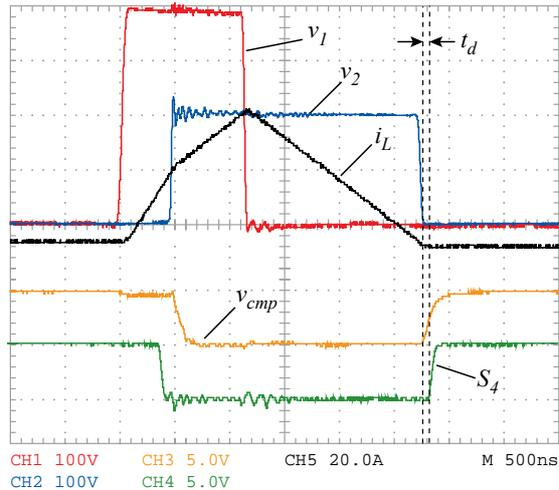
Fig 11: Ensuring ZVS by monitoring of  $S_4$  drain-source voltage  $v_2(t)$  with a comparator signal  $v_{cmp}(t)$ ; switch  $S_4$  control signal.
