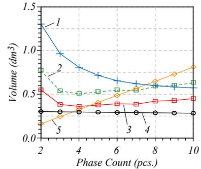
Fig. 9: Volume share of the converter sections for  $f_s = 100\text{kHz}$ , input and output filter including capacitors  $C_1$  and  $C_2$ , (1), liquid cooler (2), semiconductors (3), inductor  $L$  (4), gate drive and control circuit (5)
