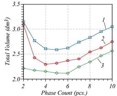
Fig. 10: Total converter volume (volume of liquid cooler not included) for switching frequencies  $f_s$  of 50 kHz (1), 100 kHz (2) and 150 kHz (3).
