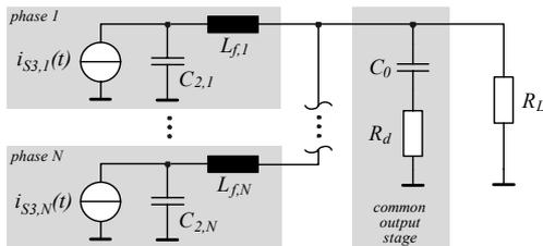
Fig. 8: Phase interconnection and input/output filter structure shown for converter side 2.
