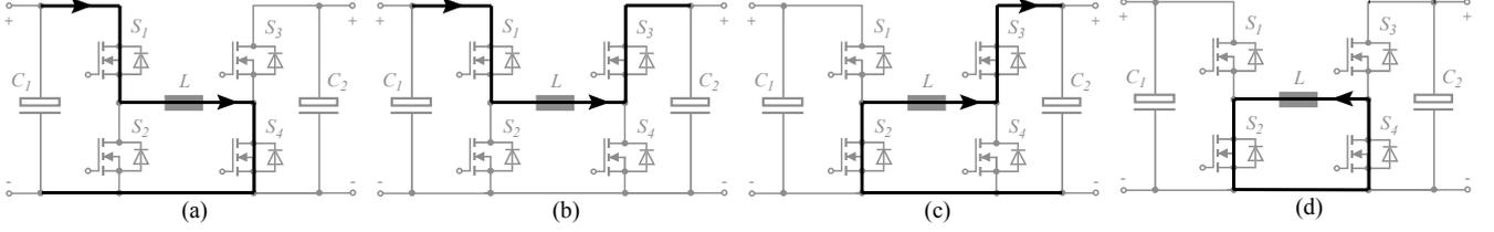
Fig. 3: Inductor current flow for time intervals  $t_0 < t < t_1$  (a),  $t_1 < t < t_2$  (b),  $t_2 < t < t_3$  (c) and  $t_3 < t < T_p$  (d). Current direction reverses in (a) and (c) as can be seen in Fig 2, which is not shown for the reason of simplicity.
