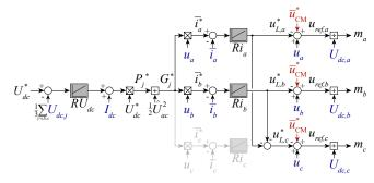
**Fig. 4.** Block diagram of a cascaded control of the PFC rectifier input stages of **Fig. 3(a)** considering a  $3^{rd}$  harmonic CM voltage injection  $\bar{u}_{\rm CM}^*$ . (Figure adapted from [1])
