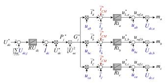
**Fig. 8.** Block diagram of a cascaded control of the PFC rectifier input stages of **Fig. 3(e)** considering a  $3^{\rm rd}$  harmonic CM current injection  $\bar{i}_{\rm CM}^*$ .
