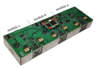
Fig. 5. Phase-modular three-phase PFC rectifier hardware prototype which can be configured for Y- and  $\Delta$ -connected operation of the modules as highlighted in Fig. 3. The system dimensions are  $395 \, \mathrm{mm} \times 125 \, \mathrm{mm} \times 50 \, \mathrm{mm}$  ( $15.6 \, \mathrm{in} \times 4.9 \, \mathrm{in} \times 2.0 \, \mathrm{in}$ ) and details on the main power components are listed in Tab. 2.
