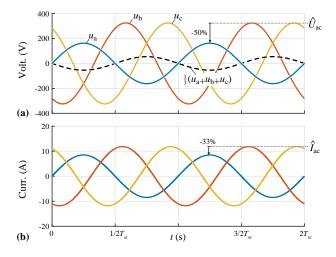
**Fig. 4.** Simulated  $3\Phi$ -ET waveforms considering the specifications of the experimental prototype system in **Sec. III** for an unbalanced grid where the input voltage of phase a shows only half the line-to-neutral amplitude of phases b and c: (a) grid input voltages  $u_{\rm a}, u_{\rm b}, u_{\rm c}$  and the CM voltage component, and (b) grid input currents  $i_{\rm a}, i_{\rm b}, i_{\rm c}$  which sum to zero in the open grid starpoint g.
