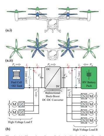
**Fig. 1.** (a) Illustration of an all-electric Vertical Takeoff and Landing (eVTOL) aircraft in (a.i) hover and (a.ii) fixed-wing cruise configuration (from [3]). (b) Considered hybrid battery-Fuel Cell (FC) power supply with an interconnecting Buck-Boost (BB) dc-dc converter regulating the power flow in between the two energy sources.
