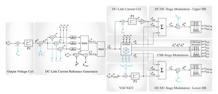
Fig. 9: Proposed control block diagram for the  $3-\Phi$  bB current DC-link PFC rectifier system shown in Fig. 3. It is based on the synergetic control concept from [20] but in addition implements virtual grounding control (VGC) or ground current control (GCC). The functionality and the interaction of the individual control blocks are described in the text. Note that all quantities refer to local average values here.
