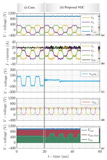
Fig. 19: Simulated key waveforms for operation in the boost-mode with distorted mains voltages (i.e., the 3- $\Phi$  mains voltages contain 12% of 5th, 10% of 7th, and 7% of 11th harmonics [44]), (i) regulated by conventional synergetic control without VGC and (ii) with the proposed VGC, where  $V_{\text{out}} = 100 \text{ V}$  and  $P_{\text{out}} = 10 \text{ kW}$ .
