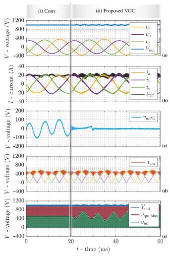
**Fig. 18:** Simulated key waveforms for operation in the boost-mode under asymmetric  $3-\Phi$  mains voltage amplitudes, e.g., +10% in phase *a* and -10% in phase *b*, (i) regulated by conventional synergetic control without VGC and (ii) with the proposed VGC, where  $V_{\text{out}} = 1000$  V and  $P_{\text{out}} = 10$  kW.
