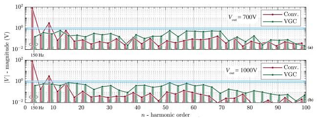
Fig. 13: Comparison of the harmonic spectra calculated from measured  $v_{mk}$  when operating without (Fig. 11) and with (Fig. 12) the proposed VGC at (a)  $V_{out} = 700 \text{ V}$ ,  $P_{out} = 4.5 \text{ kW}$  and (b)  $V_{out} = 1000 \text{ V}$ ,  $P_{out} = 9.1 \text{ kW}$ ; in all cases from a 50 Hz mains. Note that VGC successfully suppresses LF CM voltage harmonics, i.e., especially the third-harmonic component is reduced from 80 V without VGC to less than 1 V with VGC.
