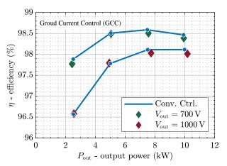
Fig. 17: Measured (Yokogawa WT3000) efficiencies of the 10 kW hardware demonstrator (see Fig. 10) with  $V_{out} = 700$  V and  $V_{out} = 1000$  V (i.e., boost-mode) and for various output power levels. Enabling GCC has almost no impact on the efficiency; and with or without GCC a high peak efficiency of about 98.5% is achieved.
