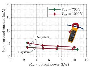
Fig. 15: Ground current  $i_{\rm GND}$  measured with a leakage current clamp meter *Fluke 368 FC* [39] for operation with two different output voltages and various power levels from 25 % to 100 % of rated load. For both grounding schemes (TT and TN), the measured ground current remains far below RCD trip levels of 30 mA.
