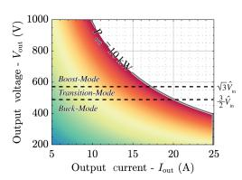
Fig. 2: Typical operating range of EV chargers, including a constant output current  $I_{out} = 25$  A region when  $V_{out} < 400$  V and a constant output power  $P_{out} = 10$  kW when  $V_{out} > 400$  V. Three operating modes, i.e., buck-mode, boost-mode and transition-mode, are required to cover such a wide output voltage range [20].
