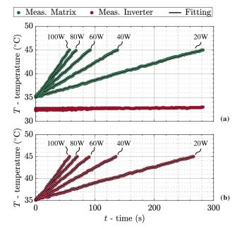
Fig. 8. Brass block calibration results for (a) matrix stage and (b) inverter stage. Note that during the calibration of the matrix stage with 20–100 W, the inverter-stage block temperatures [red in (a)] always stay at the room temperature, which confirms very good thermal insulation (decoupling) between the two brass blocks.
