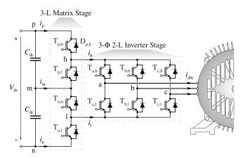
Fig. 1. Schematic of the power circuit of the three-level (3-L) sparse neutral point clamped converter (SNPCC), which is composed of a three-level 3-L matrix stage connected to a three-phase  $(3-\Phi)$  two-level (2-L) inverter stage.
