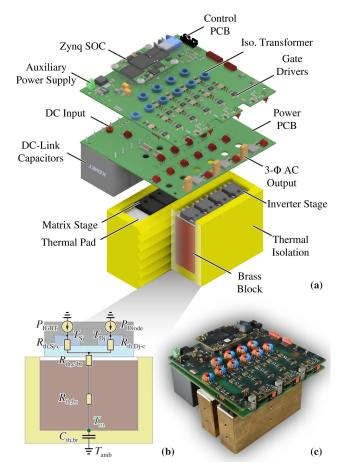
Fig. 6. (a) In-situ calorimetric semiconductor loss measurement setup, where the heat sink is replaced by two thermally insulated brass blocks to measure the matrix-stage and inverter-stage semiconductor losses, respectively. (b) Detailed equivalent thermal network for one TO-247 package (including one IGBT and one diode) and (c) photograph of the realized measurement setup.
