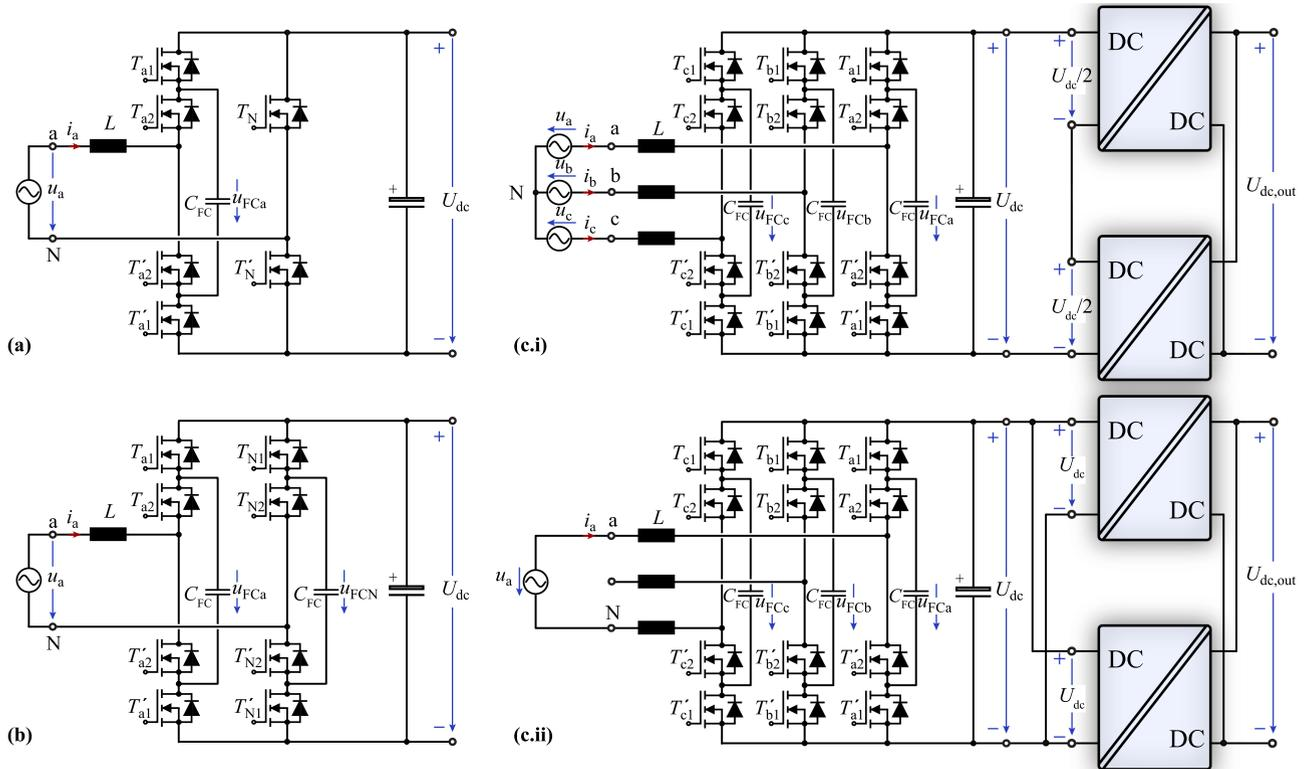
**FIGURE 8.** Further applications of the 3L FC bridge-leg with integrated PPB introduced for a single-phase PFC rectifier with a front-end diode bridge in Fig. 1: (a) bidirectional realization with a main-frequency-operated unfolded bridge-leg  $T_N/T'_N$ , (b) bidirectional H-bridge realization employing two high-frequency-operated FC bridge-legs, (c) converter topology featuring three-phase and single-phase ac-dc power conversion.
