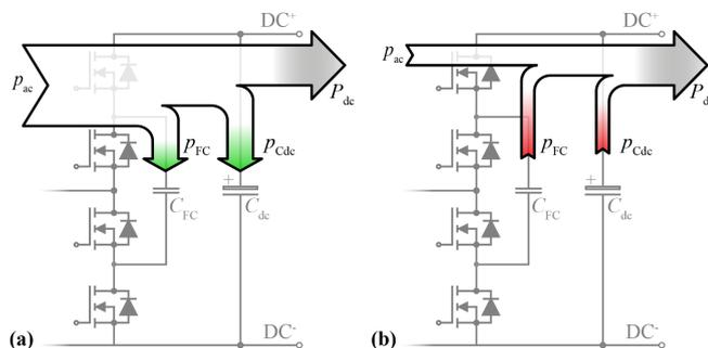
**FIGURE 2.** Sankey diagram of the main power flow quantities, i.e., grid input power  $p_{ac}$ , FC power  $p_{FC}$ , dc-link power  $p_{dc}$  and dc output power  $P_{dc}$  of a 3L FC PFC rectifier with active FC PPB operation for (a)  $p_{ac} > P_{dc}$  and (b)  $p_{ac} < P_{dc}$ , where the FC is charged and discharged, respectively in order to decrease the power pulsation of the dc-link capacitor  $p_{Cdc}$ .
