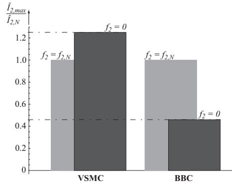
Fig.14 Calculated change in the maximum peak current for operation at nominal and zero output frequency for the VSMC and BBC. Due to various modulation strategies the VSMC can increase the output current by 25%, while for the BBC the output current must decrease by 54%.
