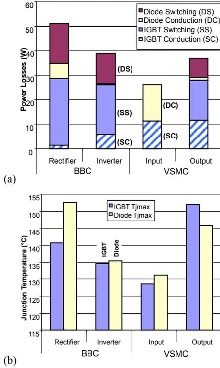
Fig.12 (a) Loss contributions and (b) junction temperatures of IGBTs and diodes at rated load for the BBC and VSMC.
