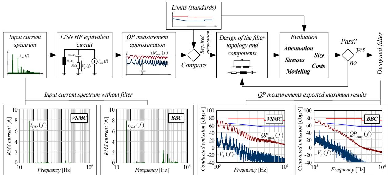
Fig.9 Filter design procedure and the input current spectra for the BBC and the VSMC, as well as the expected conducted quasi-peak emission levels measured for both systems.
