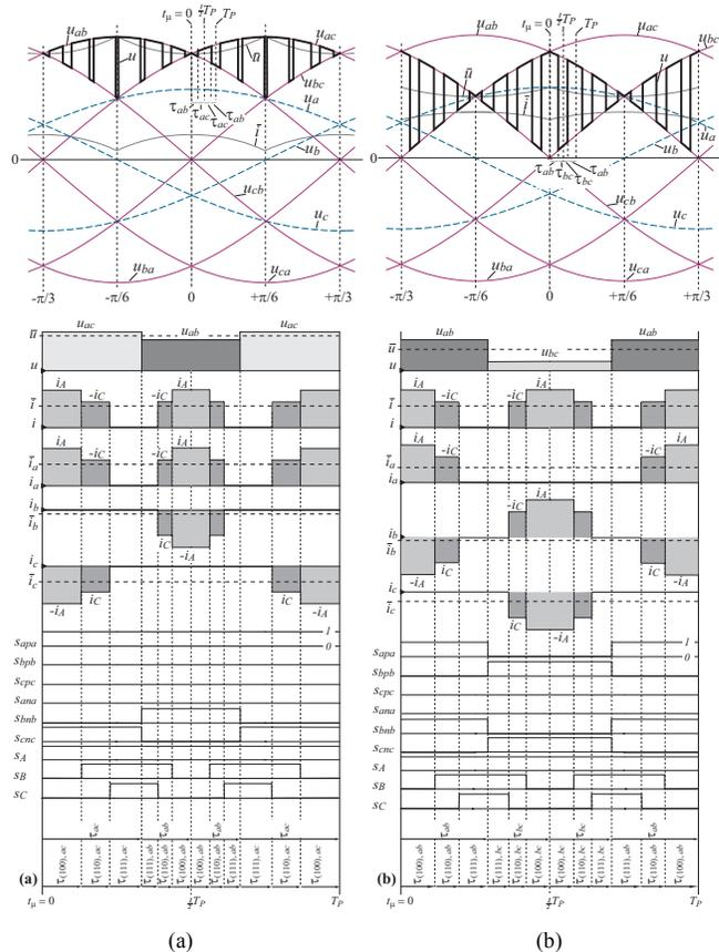
Fig.2 VSMC Modulation Schemes (a) Conventional Modulation Scheme<sup>(4)</sup>, (b) Low Output Voltage Modulation Scheme<sup>(6)</sup>. Both (a) and (b) shows the time behavior of  $u$ ,  $i$ , mains phase current  $i_1$  within a pulse period  $t_u=0 \dots T_p$  for  $\phi_1$  in  $0 \dots +\pi/6$  and  $\phi_2$  in  $0 \dots +\pi/3$  ( $\phi_1$  &  $\phi_2$  denote the phase of the reference values of the input and output voltage space vector respectively).
