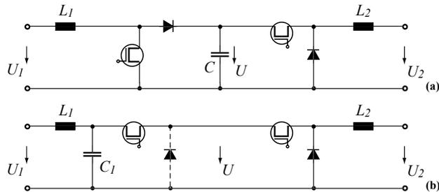
Fig.6 DC-DC equivalent circuits of the three-phase AC-AC converters (a) Back-to-Back with DC voltage link (Boost-Buck) and (b) Matrix (Buck-Buck).
