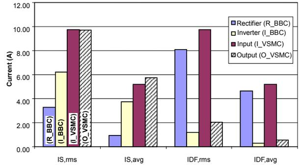
Fig.7 Current Stresses (switch rms and average, diode rms and average) for the rectifier and inverter stages of the VSMC and BBCs.
