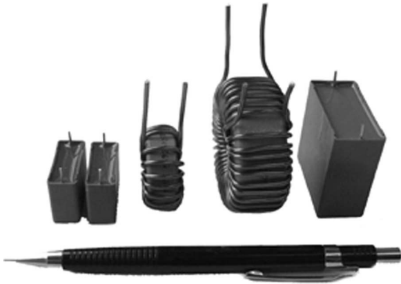
Fig. 19. Photo of main filter components (inductors and capacitors) employed for realization of designed input filter (cf., Fig. 14).
