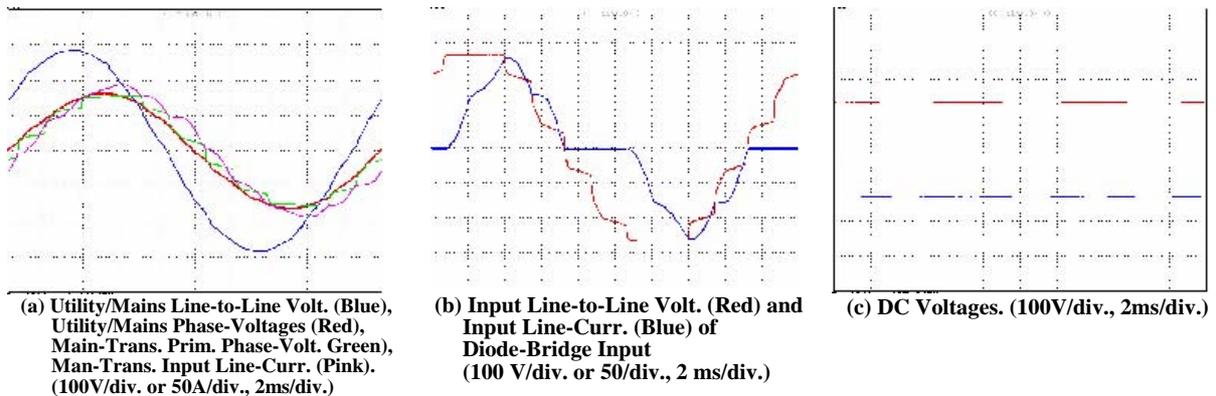
Fig. 6. Operating Waveforms of 12-Pulse Rectifier with  $L_{A,B,C}=0.784\text{mH}$
