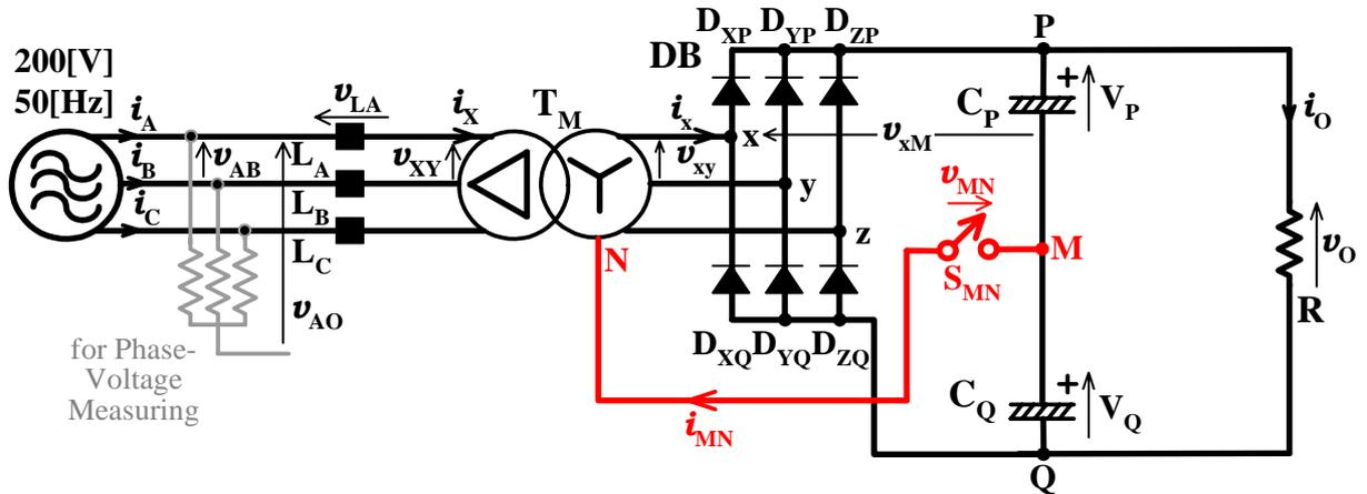
Fig. 2. Ordinary and Particular 6-Pulse Rectifiers Isolation Transformer.
