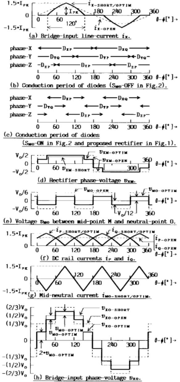
Fig. 3. Theoretical Operating Waveforms of Ordinary 6-Pulse, Particular 6-Pulse and Modified 12-pulse Rectifiers
