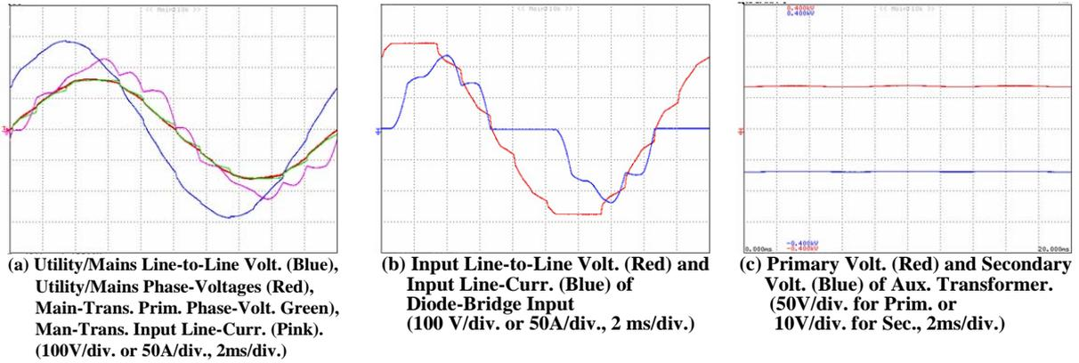
Fig. 4. Operating Waveforms of 12-Pulse Rectifier with  $L_{A,B,C}=0.217\text{mH}$
