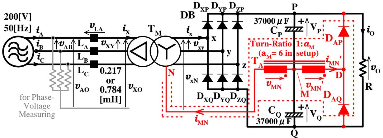
Fig. 1. Modified 12-Pulse Rectifier with Isolation Transformer.
