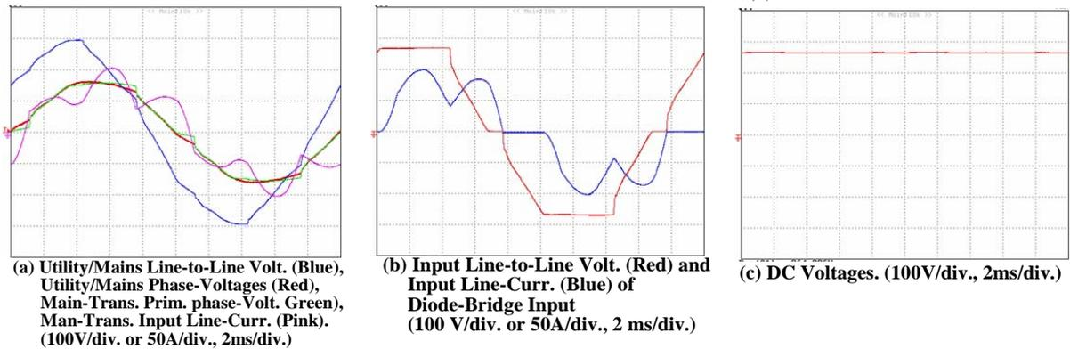
Fig. 5. Operating Waveforms of 6-Pulse Rectifier with  $L_{A,B,C}=0.217\text{mH}$
