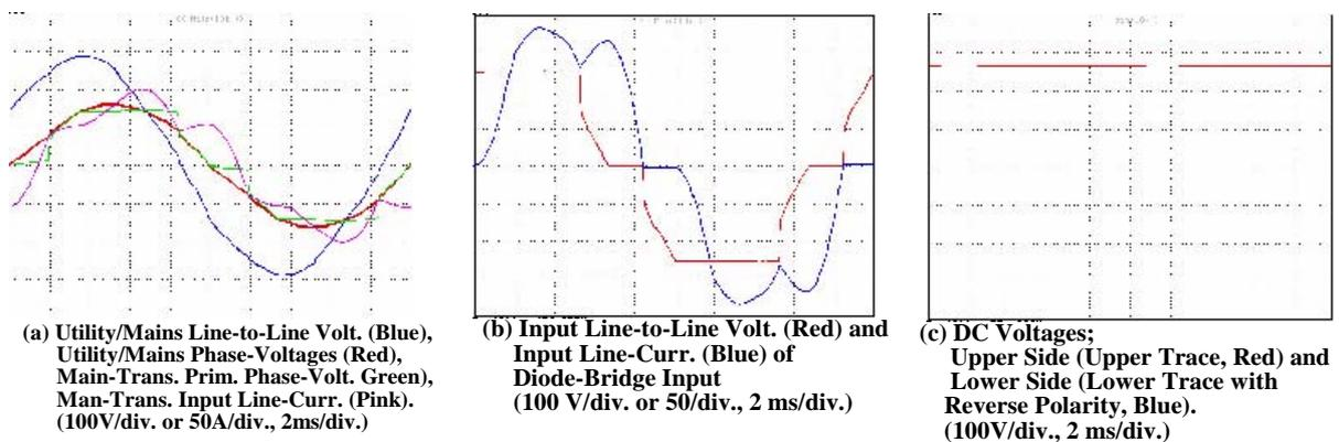
Fig. 7. Operating Waveforms of 6-Pulse Rectifier with  $L_{A,B,C}=0.784\text{mH}$
