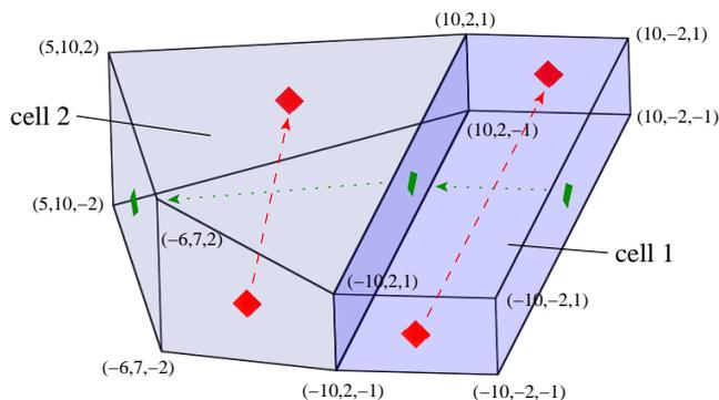
Fig. 4. Example cell geometry: two inductive PEEC cells. Two different current directions (dashed and dotted) and the cell corner point coordinates are given (in mm) so that numeric results are replicable.
