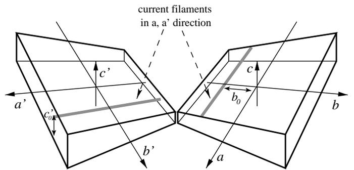
Fig. 2. Two inductive hexahedral PEEC volume cells with current direction  $a$  and  $a'$ . The coordinate axes indicate a local non-orthogonal coordinate system, as introduced in [4]. Furthermore, two current filaments, pointing respectively in  $a$  and  $a'$  direction, are displayed.
