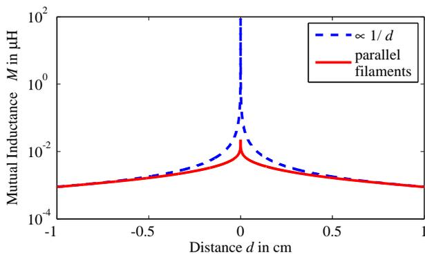
Fig. 3. Mutual inductance between two parallel current filaments of length  $l = 1$  cm. Approaching a zero distance  $d$ , the inductance  $M$  is diverging to infinity. However, the divergence  $\propto \log(2l/r)$  is relatively weak in comparison to the  $1/d$  Green's function, which allows a more efficient numeric integration of the partial elements.
