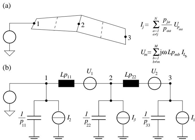
Fig. 1. Two non-orthogonal conductor cells (a) and their corresponding equivalent circuit (b).
