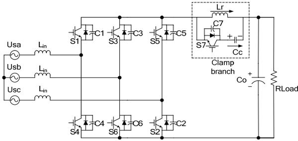
Fig.1. ZVS-SVM controlled active-clamp three-phase boost rectifier
