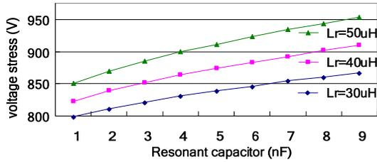
Fig.7 Voltage stress vs. resonant parameter (simulation result)
