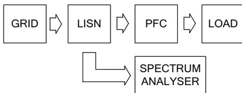
Fig.5 Circuit connection of the conducted emission measurement
