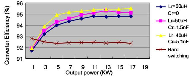
Fig.9 Efficiency vs. Po with different resonant components parameters (fs=50kHz) (experimental results)
