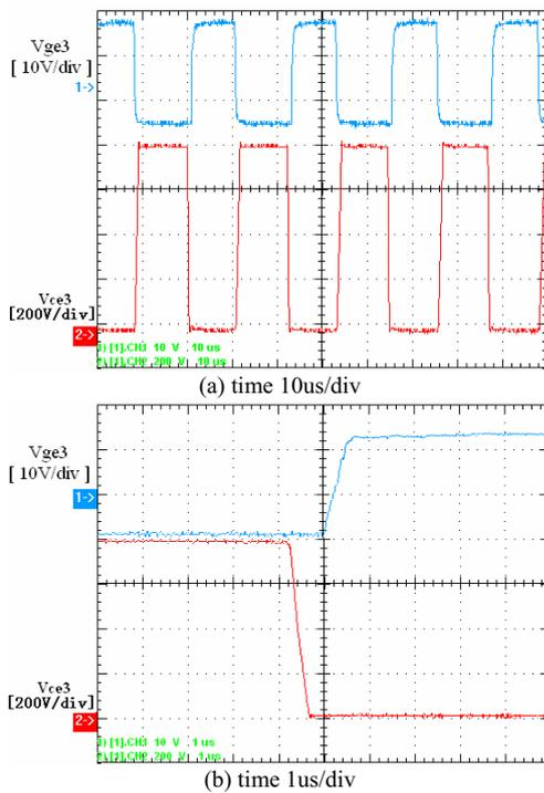
Fig. 13 CE voltage and driving signal of the main switch S3
