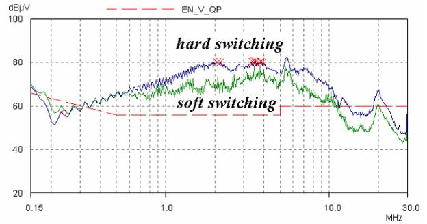
Fig.6. Comparison of conducted EMI in hard switching and soft switching conditions
