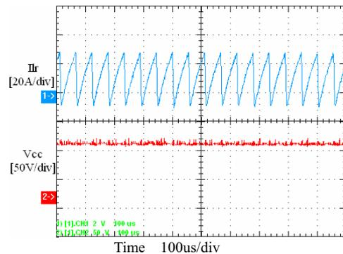
Fig. 15 Current of Lr and voltage on clamping capacitor
