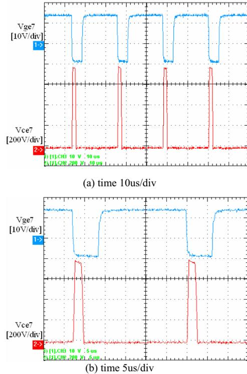
Fig.14 CE voltage and driving signal of the auxiliary switch S7
