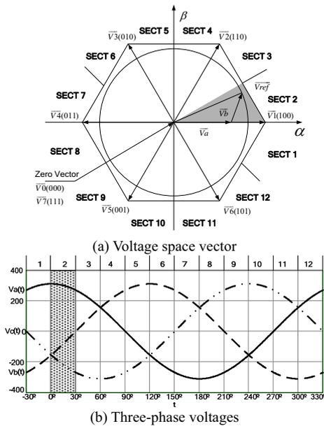
Fig.2. Three-phase voltages and voltage space vectors
