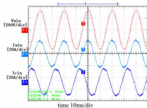
Fig. 11 Input voltage and current
