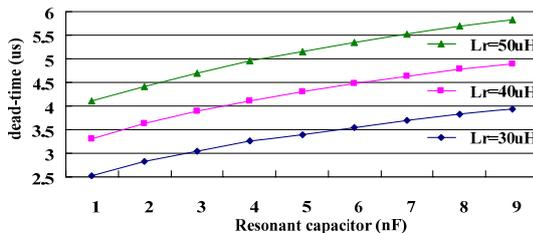
Fig.8 switching dead-time vs. resonant parameter (simulation results)
