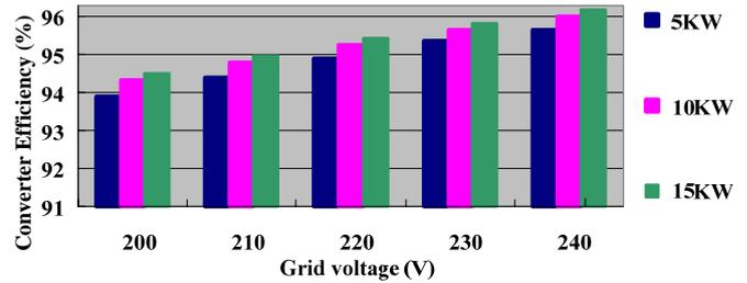
Fig.10 Efficiency vs. Uin with different output load (fs=50kHz) (experimental results)
