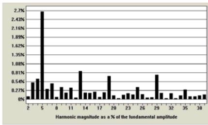
Figure 12. Input current harmonic spectrum
