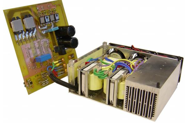
**Fig.7:** Prototype of a 10kW TSHR; overall dimensions:  $24.0 \times 22.9 \times 11.7 \text{cm}^3$
