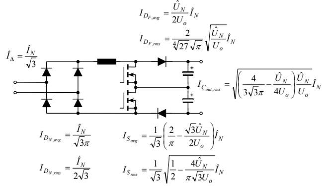
**Fig.6:** Circuit structure of a line-to-line module of the  $\Delta$ -Rectifier and current stresses on the power components according to (20) – (27).
