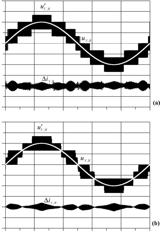
**Fig. 4:** Time behavior of a mains phase voltage  $u_{N,R}$ , of the equivalent rectifier input phase voltage  $u'_{N,R}$  (cf. Fig. 2 in [2]) and of the current ripple  $\Delta i_{N,R}$  of the mains phase current  $i_{N,R}$  of the conventional rectifier (cf. (a)) and of the  $\Delta$ -Rectifier (cf. (b)).
