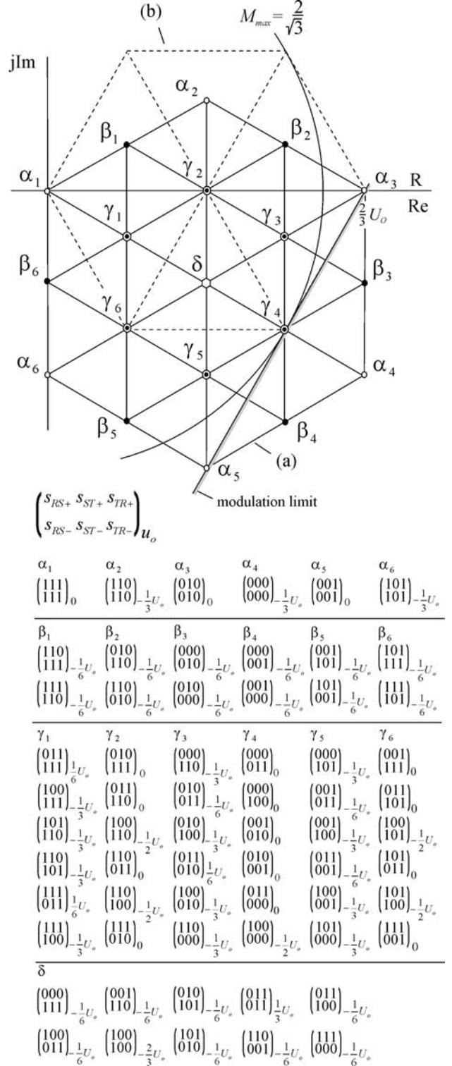
**Fig.2:** Voltage space vectors available for input current control; (a) three-level  $\Delta$ -Rectifier, (b) conventional rectifier (cf. Fig. 4 in [1]).
