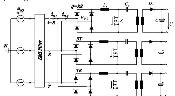
Fig.8: Basic structure of the power circuit of a SEPIC-type  $\Delta$ -Rectifier [11].
