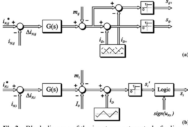
**Fig. 3:** Block diagram of the input current control of a line-to-line module of a three-level  $\Delta$ -Rectifier (cf. (a)) and phase current control of a conventional rectifier (cf. (b)).
