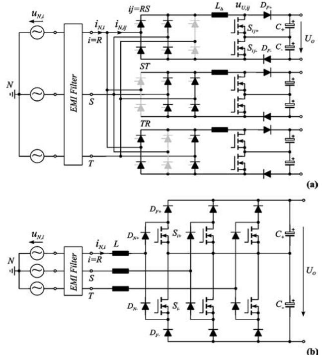
**Fig.1:** Basic structure of the power circuits of three-phase boost-type unity power factor rectifiers; **(a):** delta connection of single-phase modules ( $\Delta$ -Rectifier), or **(b)** direct three-phase realization as proposed in [3] (denominated as *conventional* rectifier in the following).
