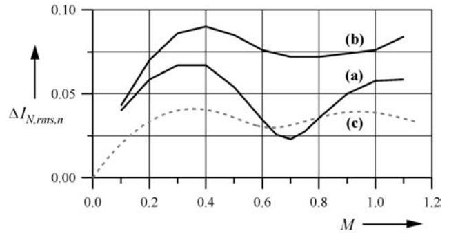
**Fig.5:** Normalized rms value  $\Delta I_{N,rms,n}$  of the phase current of the three-level  $\Delta$ -Rectifier (cf. (a)) and of a conventional rectifier (cf.(b)). Furthermore shown: rms value of the ripple  $\Delta I_{N,ij,rms,n}$  of the input current of a line-to-line module of a  $\Delta$ -Rectifier (cf.(c)) as used for the calculation of the inductor core losses.
