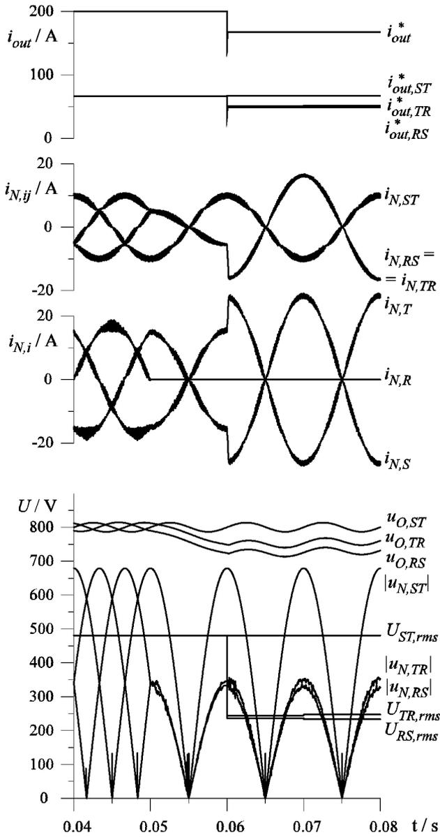
**Fig.4:** Section of the overall time behavior shown in Fig.3 around the instant in time where the mains phase R loss does occur ( $t = 50\text{ms}$ ). Special attention has to be paid to the measurement of the rms values of the mains voltages which is delayed by 10ms in order to perform the rms value calculation.
