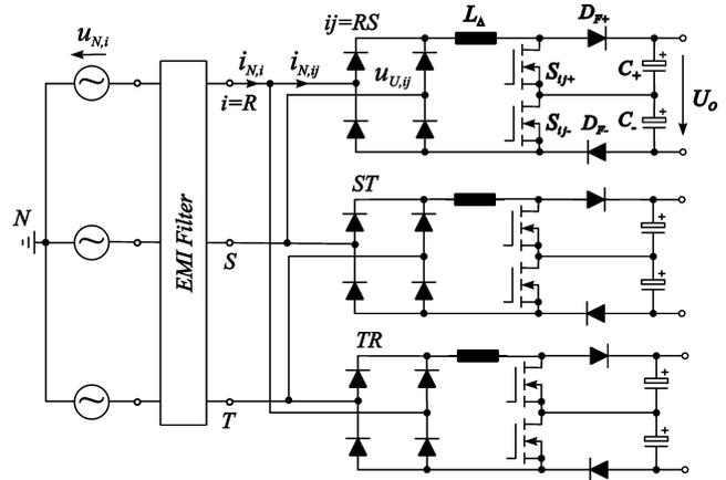
**Fig.1:** Basic structure of the power circuit of a three-phase boost-type unity power factor rectifier formed by input-side delta-connection of three single-phase three-level power factor corrected rectifier modules (three-level  $D$ -Rectifier).
