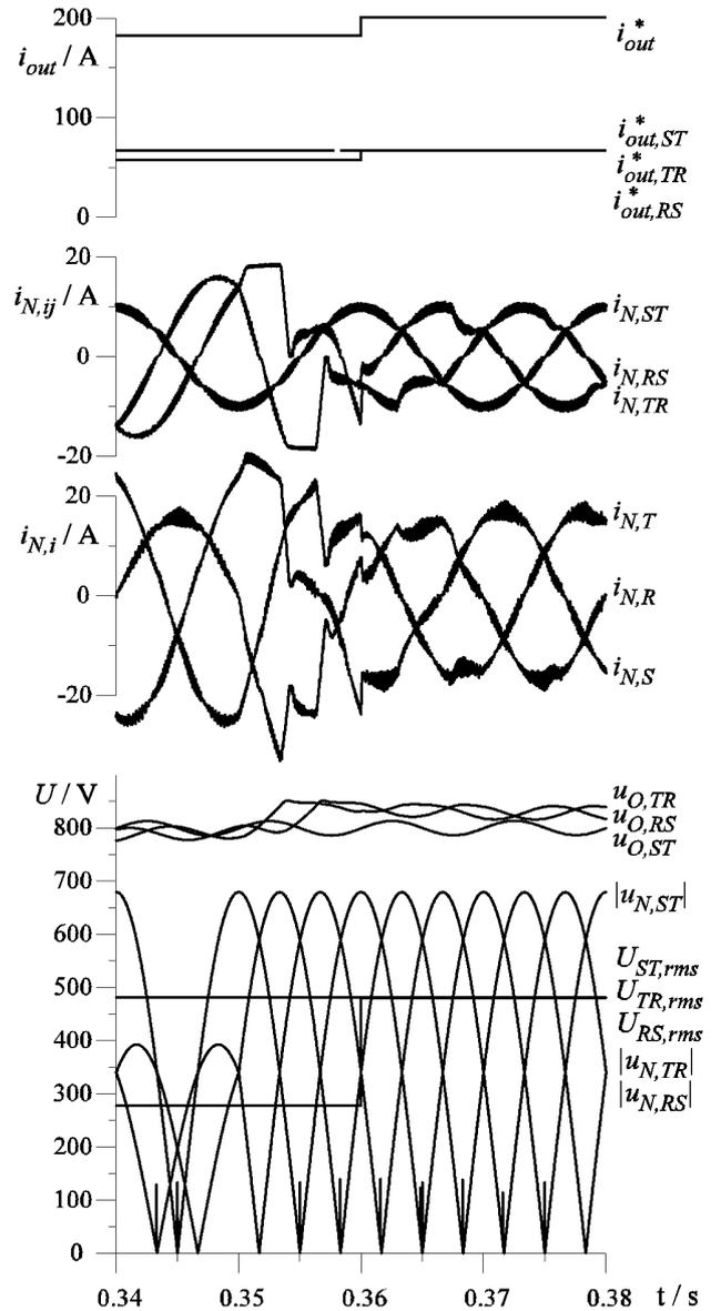
**Fig.7:** Section of the time behavior shown in Fig.3 around the instant in time where the mains phase R earth fault is removed ( $t = 350\text{ms}$ ). Special attention has to be paid to the current limit of the line-to-line currents  $i_{N,RS}$  and  $i_{N,TR}$  and the rail voltage limit of  $u_{O,RS}$  and  $u_{O,TR}$  where the actual rms value of the line-to-line voltage is not yet calculated correctly.
