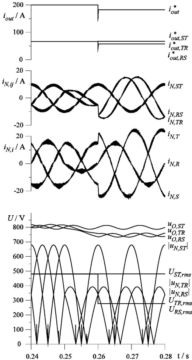
**Fig.6:** Section of the time behavior shown in Fig.3 around the instant in time where the mains phase R earth fault does occur ( $t = 250\text{ms}$ ). Special attention again has to be paid for the calculation of the rms values of the mains line-to-line voltages which does cause a delay of 10ms in the conductance calculation.
