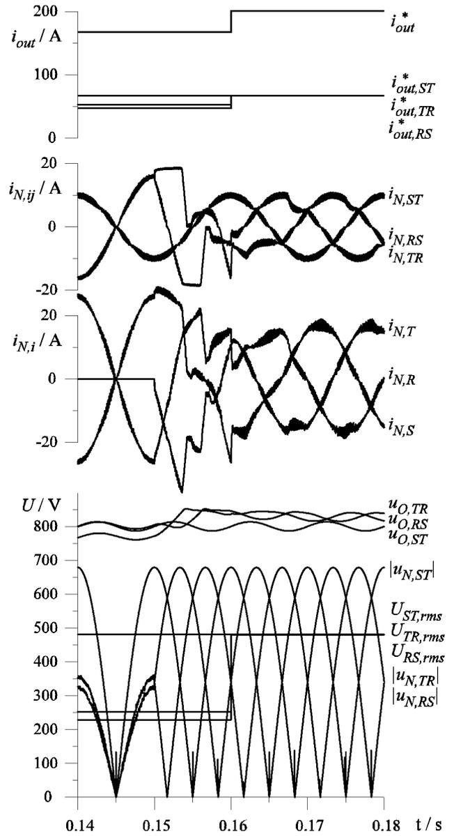
**Fig.5:** Section of the overall time behavior shown in Fig.3 around the instant in time where the mains phase R does return ( $t = 150\text{ms}$ ). Special attention has to be paid to the current limit of the line-to-line currents  $i_{N,RS}$  and  $i_{N,TR}$  and to the rail voltage limit of  $u_{O,RS}$  and  $u_{O,TR}$  where the actual rms value of the line-to-line voltage temporarily is calculated incorrectly.
