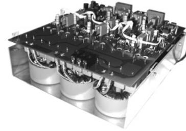
**Fig.31:** Prototype of a 10kW SMC. The system control (not shown) is realized by a DSP in combination with programmable logic devices. The overall dimensions of the system including the input filter are  $24 \times 20 \times 8.5\text{cm}^3$  resulting in a power density of  $\rho=2.5\text{kW/dm}^3$ .
