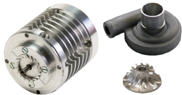
Figure 2. PM generator with stator guide vanes, spiral casing and radial turbine ( d = 10.5 \text{ mm} ).
