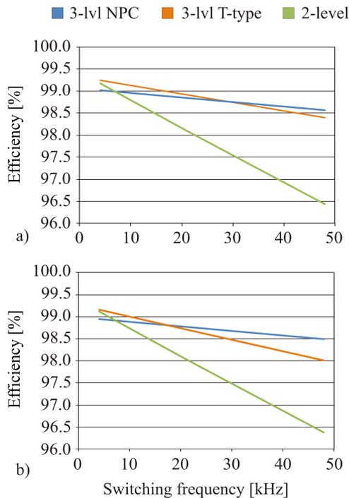
Fig. 4. Efficiency comparison between the different topologies. a) Rectifier operation with  $\hat{U} = 325$  V,  $\hat{I} = 21.5$  A,  $\phi_1 = 180^\circ$ , b) inverter operation with  $\hat{U} = 325$  V,  $\hat{I} = 21.5$  A,  $\phi_1 = 0^\circ$ . Switch types: Infineon IKW25T120 and IKW30N60T.
