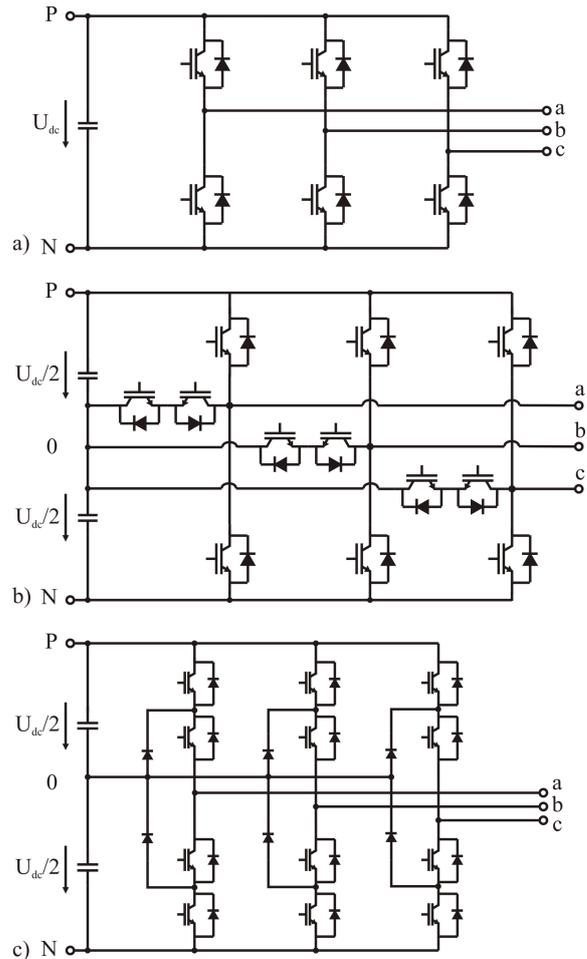
Fig. 1. Topologies of the a) 2-level, b) 3-level T-type and c) 3-level NPC voltage source converters.
