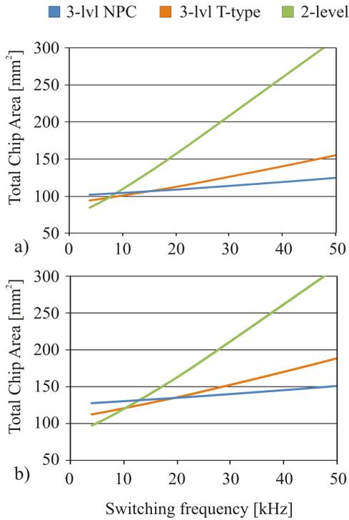
Fig. 7. Comparison of the total semiconductor area depending on the frequency. a) Rectifier operation, b) inverter operation.
