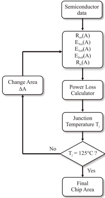
Fig. 6. Diagram of chip area optimization algorithm.
