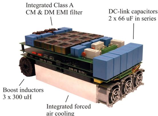
Fig. 3. 3-level NPC back-to-back converter prototype.
