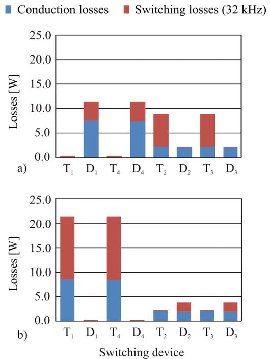
Fig. 5. Mean loss distribution in the T-type topology elements for a) rectifier operation, b) inverter operation.
