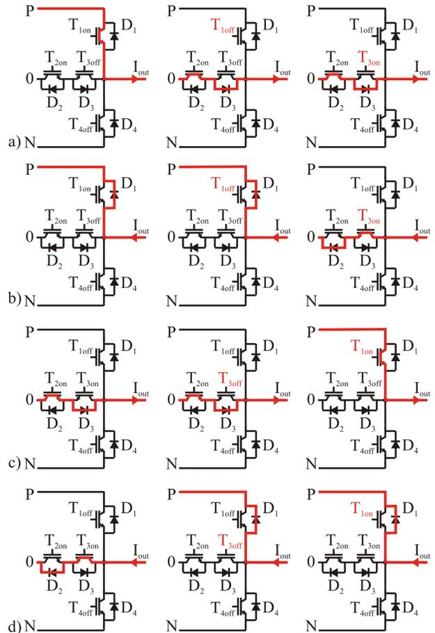
Fig. 2. Current commutation during switching transition (P  $\rightarrow$  0) for a) positive and b) negative output current. Current commutation during switching transition (0  $\rightarrow$  P) for c) positive and d) negative output current.
