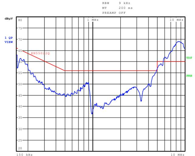
Fig.14: Measured conducted emission levels at a DM output of the three-phase CM/DM noise separator.
