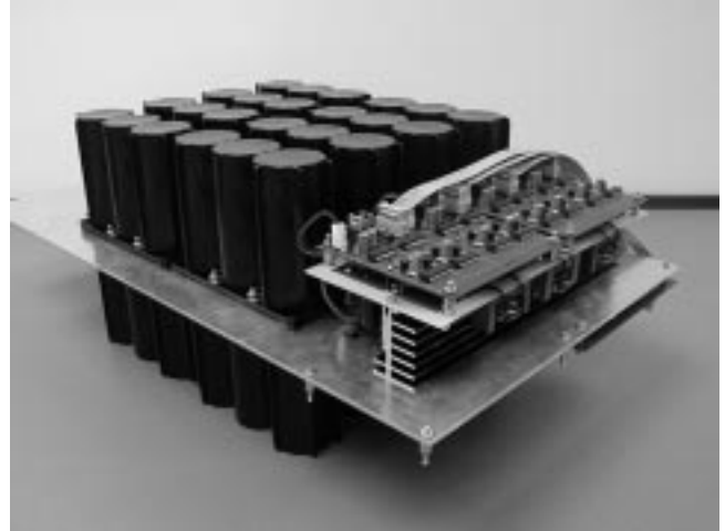
Fig. 11. “Flying-battery” amplifier laboratory setup.
