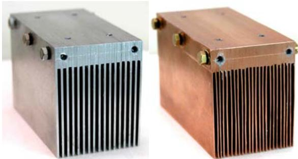
Fig.6. Sub-optimum stacked heat sinks employing SanAce40/50dB (not shown) with  $b=c=40mm$ ,  $d=10mm$ ,  $L=80mm$ ,  $A_{CHIP}=32cm^2$ ,  $Vol_{CS}=0.4 \times (0.4+0.1) \times (0.80+0.05+0.28)=0.226$  liter. (a) Aluminum with  $n=16$ ,  $s=1.5mm$ ,  $t=1.0mm$ ,  $R_{th}=0.26$ . (b) Copper with  $n=23$ ,  $s=1.3mm$ ,  $t=0.5mm$ ,  $R_{th}=0.22$ .
