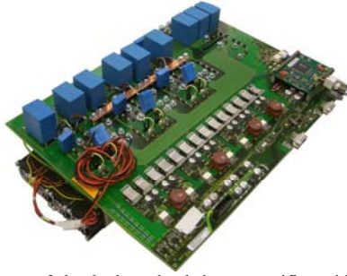
Figure 3: Photo of the 3-phase buck boost rectifier with unity power factor and a wide input and output range.
