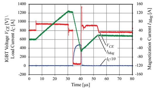
Fig. 10: Asymmetric flux swing, where  $T_{Premag} > T_{Demag}$
