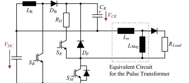
Fig. 6: Schematic of the measurement setup for the active premagnetization and the DC/DC supply.
