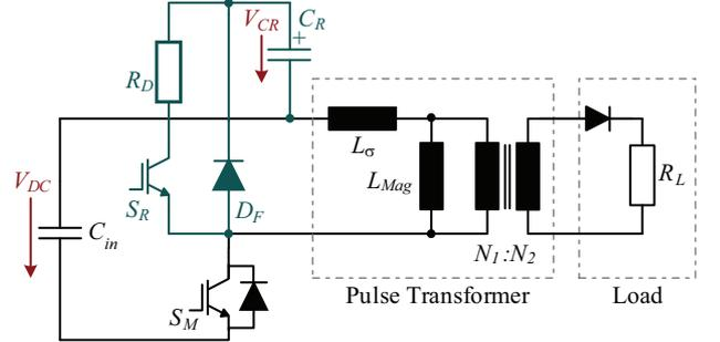
Fig. 2: Schematic of the pulse modulator with the active reset circuit.
