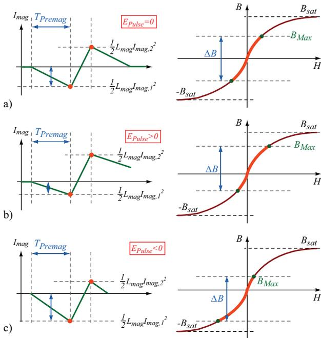
Fig. 5: **a)**  $I_{Mag,1} = \frac{1}{2}\Delta I_{Mag}$ : The energies after and before the pulse are the same, **b)**  $I_{Mag,1} < \frac{1}{2}\Delta I_{Mag}$ : The energy after the pulse is the higher than the energy before the pulse and **c)**  $I_{Mag,1} > \frac{1}{2}\Delta I_{Mag}$ : The energy after the pulse is the lower than the energy before the pulse .
