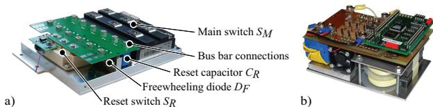
Fig. 8: a) Prototype of the active reset circuit and b) DC/DC boost converter ( $V_{in} = 1000V$ ,  $V_{out} = 0...200V$ ,  $P_{out} = 1kW$ ).
