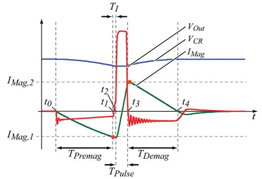
Fig. 4: Current and voltage waveforms for the active premagnetization for one pulse period.
