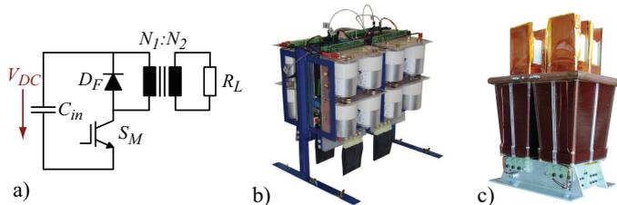
Fig. 1: a) Schematic a solid state power modulator, b) Pulse generator unit with four parallel connected IGBT modules and c) step up pulse transformer.
