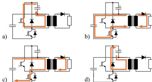
Fig. 3: Current paths during a) the premagnetization time  $T_{P_{\text{premag}}}$ , b) the interlocking delay  $T_I$ , c) the pulse duration  $T_{P_{\text{pulse}}}$  and d) the demagnetization time  $T_{D_{\text{demag}}}$ .
