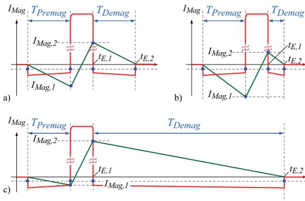
Fig. 7: a) Symmetric flux swing, where  $T_{Premag} = T_{Demag}$ , b) and c) asymmetric flux swing, where  $T_{Premag} > T_{Demag}$  respectively  $T_{Premag} < T_{Demag}$ .
