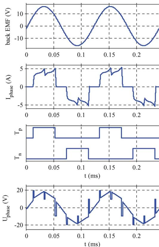
Fig. 7. Simulation of the drive system at 500 000 r/min with a VSI with block commutation an additional dc–dc converter ( $f_{\text{dcdc}} = 100 \text{ kHz}$ ,  $L_{\text{dcdc}} = 50 \mu\text{H}$ ). Machine back EMF, phase current, half-bridge switching signals and phase voltage for one phase are shown. The inverter switching frequency is the fundamental frequency of the machine (8.3 kHz).
