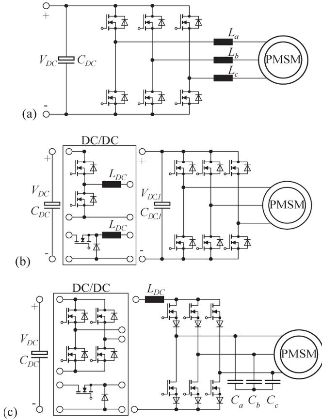
Fig. 5. Possible Power Electronic Interfaces: (a) VSI with external inductances, (b) VSI for block commutation and (c) CSI with external capacitors. Switching at fundamental frequency (8.3 kHz) the VSI (b) and CSI (c) need an additional dc–dc converter, either (top) bidirectional for motor and generator operation or (bottom) unidirectional for motor only operation.
