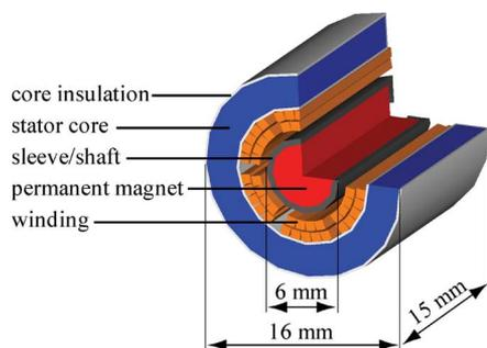
Fig. 3. Cross section of the slotless brushless PM generator. The machine has a total volume of  $3.5 \text{ cm}^3$ .
