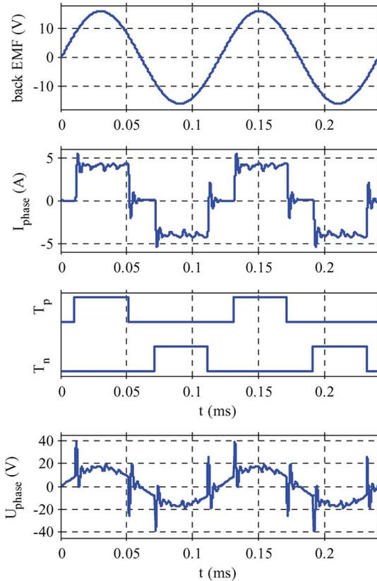
Fig. 8. Simulation of the drive system at 500 000 r/min with a CSI with block commutation an additional dc–dc converter ( $f_{dc/dc} = 100$  kHz,  $L_{dc/dc} = 100$   $\mu$ H). Machine back EMF, phase current, half-bridge switching signals and phase voltage for one phase are shown. The inverter switching frequency is the fundamental frequency of the machine (8.3 kHz).
