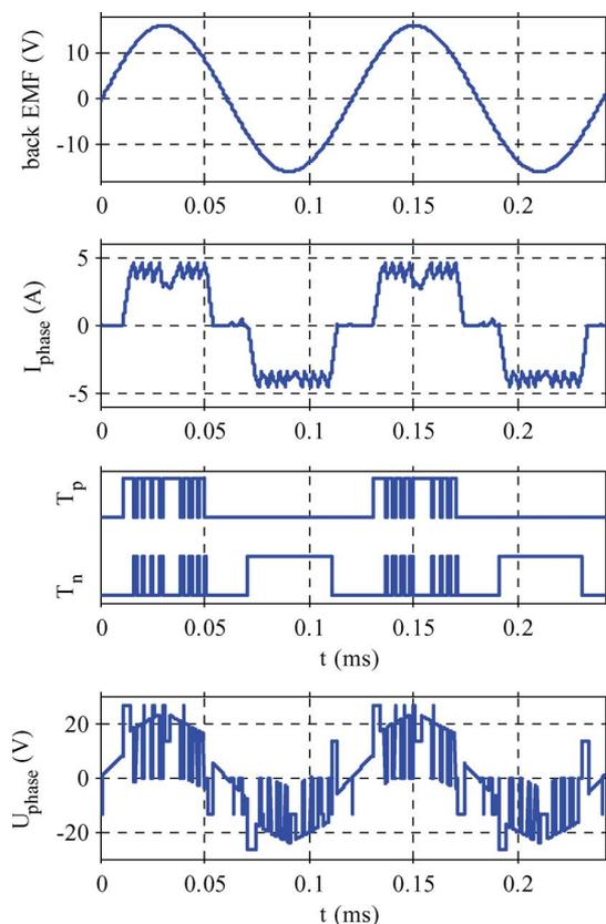
Fig. 6. Simulation of the drive system at 500 000 r/min with a VSI and additional external inductances ( $L_a = L_b = L_c = 10 \mu\text{H}$ ,  $V_{\text{DC}} = 40 \text{ V}$ ). Machine back EMF, phase current, half-bridge switching signals and phase voltage for one phase are shown. The switching frequency is approximately  $f_s = 230 \text{ kHz}$ .
