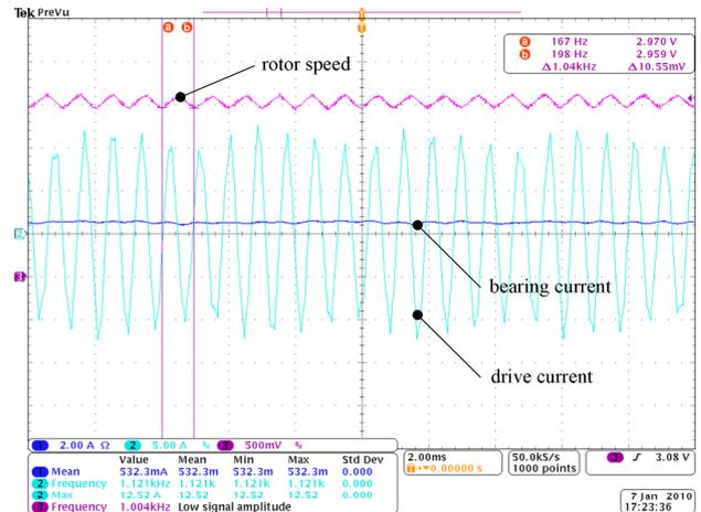
Fig. 4. Rotor ( $d = 4$  mm, with passive damping by damping needle) stably spinning at 60'000 rpm.
