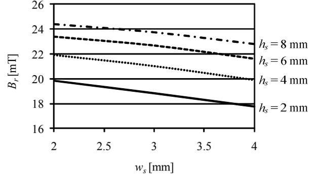
Fig. 7. Magnetic field density  $B_r$  in the rotor depending on the inner coil dimensions  $w_s$  and  $h_s$  ( $l_d = 15 \text{ mm}$ ,  $h_d = 9 \text{ mm}$ ,  $J_d = 3 \text{ A/mm}^2$ ).
