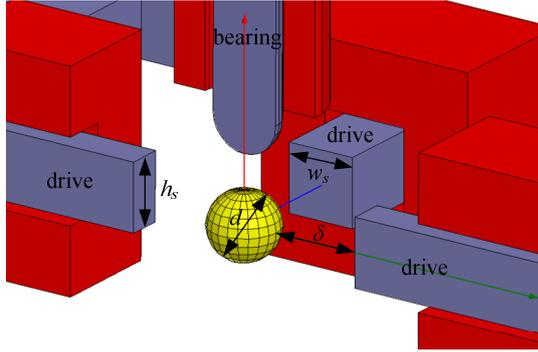
Fig. 2. Parameters describing the configuration of the first prototype.
