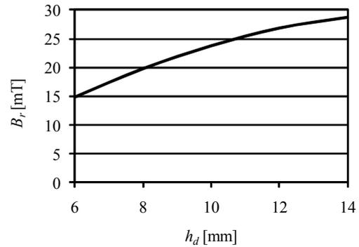
Fig. 9. Magnetic field density  $B_r$  in the rotor depending on the drive coil height  $h_d$  ( $w_s = 2 \text{ mm}$  and  $h_s = 4 \text{ mm}$ ,  $l_d = 15 \text{ mm}$ ,  $J_d = 3 \text{ A/mm}^2$ ).
