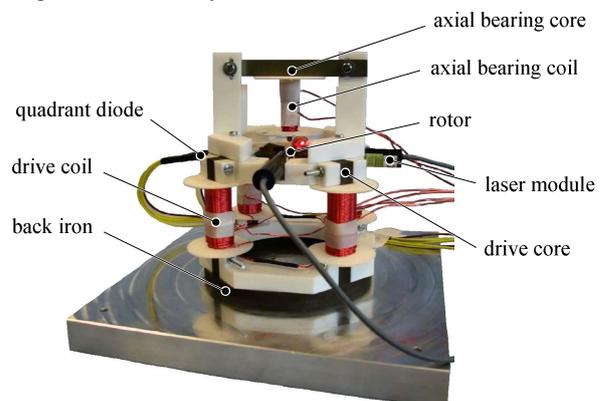
Fig. 1. First preliminary test setup of the ultra-high speed motor.
