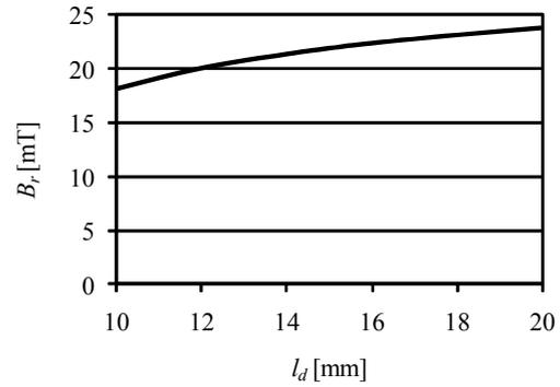
Fig. 8. Magnetic field density  $B_r$  in the rotor depending on the drive coil length  $l_d$  ( $w_s = 2 \text{ mm}$  and  $h_s = 4 \text{ mm}$ ,  $h_d = 9 \text{ mm}$ ,  $J_d = 3 \text{ A/mm}^2$ ).
