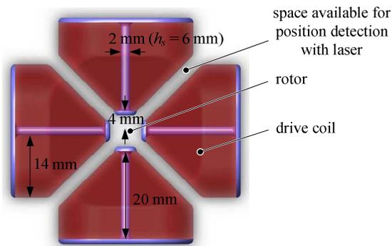
Fig. 10. Coreless drive geometry of the second prototype.
