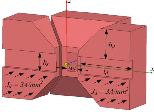
Fig. 6. Cross-section of the setup showing the parameters used for the drive unit optimization for the final setup ( $d = 1 \text{ mm}$ ).
