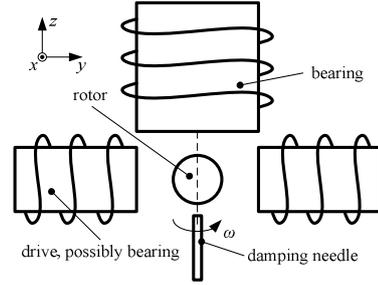
Fig. 3. Schematic setup to control all degrees of freedom and still defining a preferred position of the rotor in the motor center by using a damping needle below the rotor.
