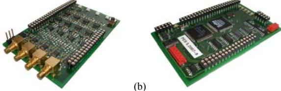
**Figure 10:** (a) Photo of the signal processing electronics and (b) of the DSP/FPGA board (credit card size for both boards: 86mm x 54mm).
