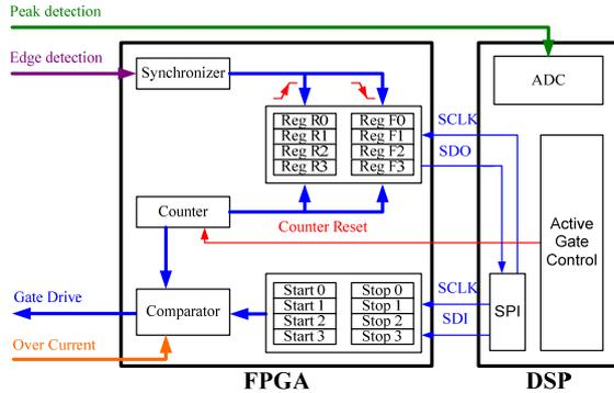
**Figure 11:** Block schematic of the implemented active gate controller in the DSP/FPGA. There, the detection of the pulse falling and rising edges, the detection of the peak values and the generation of the gate signals is shown.
