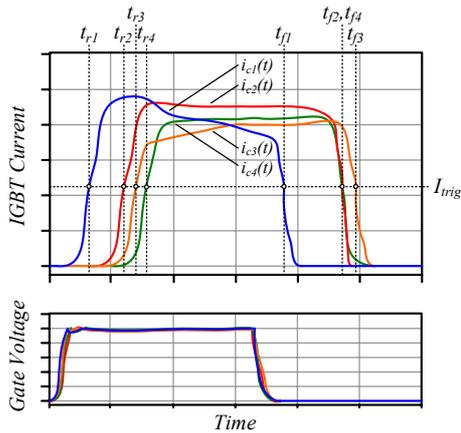
**Figure 4:** Schematic example for unbalanced current waveforms without *rise and fall time control* showing rise and fall time detection at the trigger level  $I_{trig}$ .
