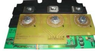
**Figure 8:** IGBT Module (single switch) with three PCB Rogowski coils, where one coil encloses one (Emitter-) terminal of the IGBT. The coils are connected in series for measuring the total switch current.
