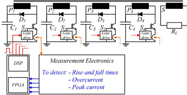
**Figure 3:** Block diagram of the modulator with active gate control.
