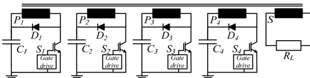
**Figure 1:** Schematic of the solid state modulator with four paralleled IGBT modules and pulse transformer with four primary windings and one secondary winding.
