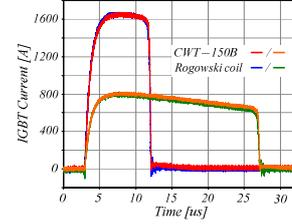
**Figure 12:** Comparison of the measurement results of the PCB-Rogowski to the results obtained with a commercial CWT-150B from PEM.
