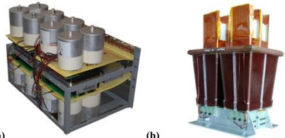
**Figure 2:** Solid state modulator: (a) Four 3.6kA-IGBT Modules plus capacitors/freewheeling diode connected to corresponding primary windings of the pulse transformer in (b).
