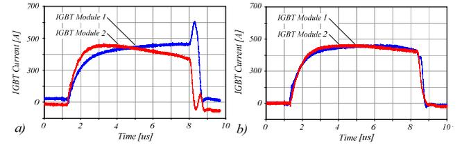
**Figure 13:** Current distribution in two direct parallel connected IGBT modules (Eupec FZ3600R17KE3) without (a) and with active gate control (b).
