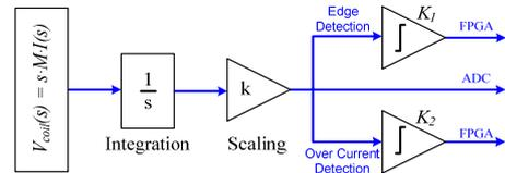
**Figure 9:** Block schematic of the measurement and signal processing electronic with edge detection  $K_1$ , over current shutdown and peak value measurement  $K_2$ .
