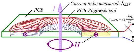
**Figure 7:** Measuring principle with a PCB-Rogowski coil.
