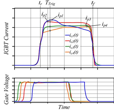
**Figure 5:** Schematic examples for IGBT current pulses with synchronized rising and falling edges based on shifted gate signals. Furthermore, the detection of the current amplitudes at the time  $T_{Trig}$  and the peak currents  $i_{pi}$  are shown.
