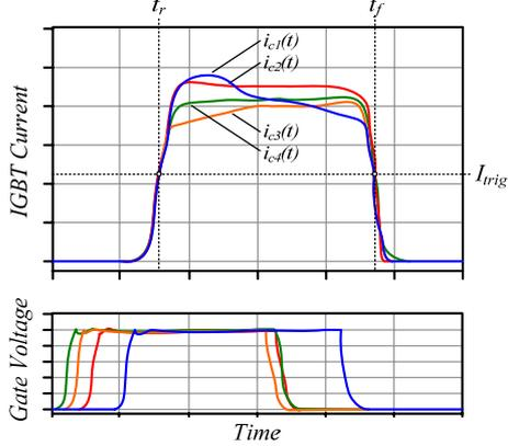
**Figure 6:** Schematic example for IGBT current pulses with synchronized rising/falling edge and synchronized slope of the rising current edge.
