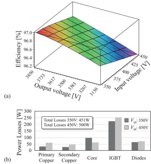
Figure 8: (a) Efficiency of the converter in the whole input and output voltage range and (b) loss distribution for the two operating points  $V_{in} = 350$  V,  $V_{out} = 3850$  V and  $V_{in} = 450$  V,  $V_{out} = 3850$  V at maximum output power.
