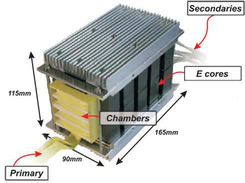
Figure 7: Final transformer: Height: 115 mm, Width: 90 mm, Length: 165 mm.
