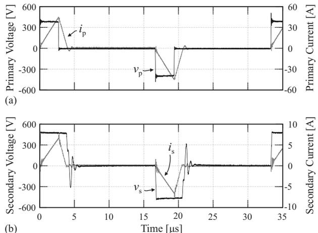
Figure 10: Experimental waveforms: (a) Primary voltage and current; (b) Voltage and current of one secondary.
