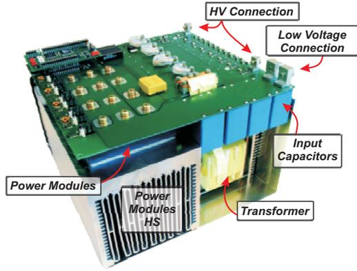
Figure 6: Picture of the designed 3.5 kV/11 kW isolated full-bridge based DC-DC converter.
