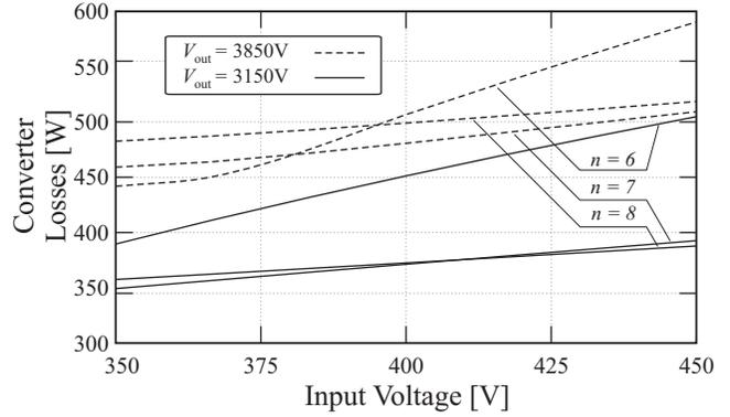
Figure 5: Overall losses for different output voltages and turns ratio.
