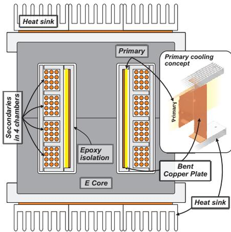
Figure 4: Cross sectional view of the transformer.
