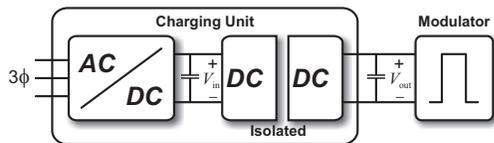
Figure 1: Block diagram of the charging unit, consisting of a three-phase AC-DC and a DC-DC converter, which interconnects the power modulator to the mains.
