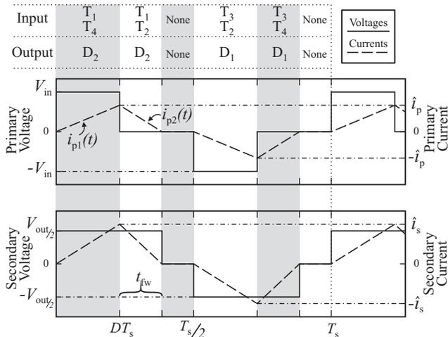
Figure 3: Qualitative operation waveforms of the full-bridge based DC-DC converter.
