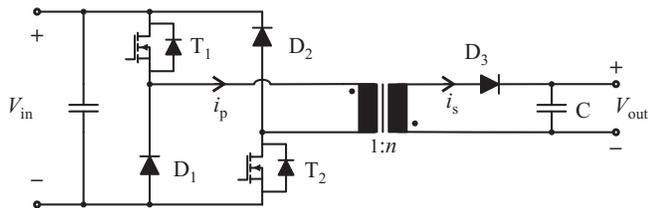
Figure 9: Schematic of the two switch flyback converter.
