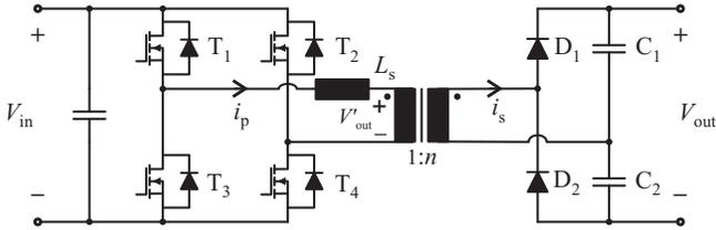
Figure 2: Schematic of the isolated, full-bridge based DC-DC converter.
