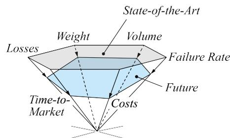
Fig. 1 State-of-the-art and future performance improvement of power electronic systems.
