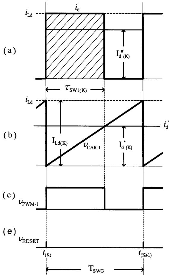
**Fig. 3. Operating Waveforms of Pulse-Integral-Value Modulation for Buck-Mode Operation.**
