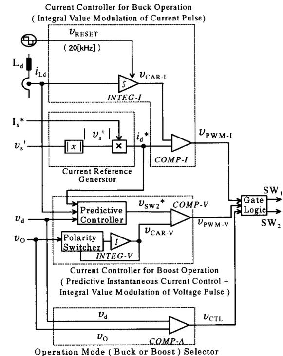
**Fig. 2. Current Controller for Dual-Switch Single-Phase PFC Rectifier with Buck-Mode and Boost-Mode Hybrid Operation.**
