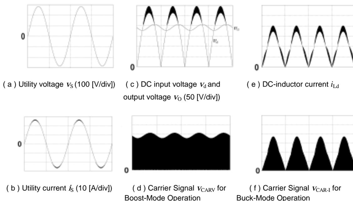
**Fig.4. Operating Waveforms of New PFC Rectifier (obtained from simulation ).**
