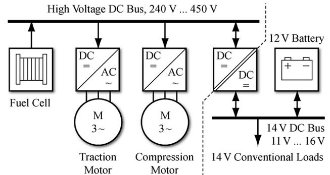
Fig. 1. Fuel cell car system architecture proposed in [3]; the fuel cell is directly connected to an HVDC bus and provides power to the traction motor and the fuel compression motor. A bidirectional dc–dc converter is employed to enable arbitrary power transfer between the HVDC bus and the conventional 14 V dc bus.
