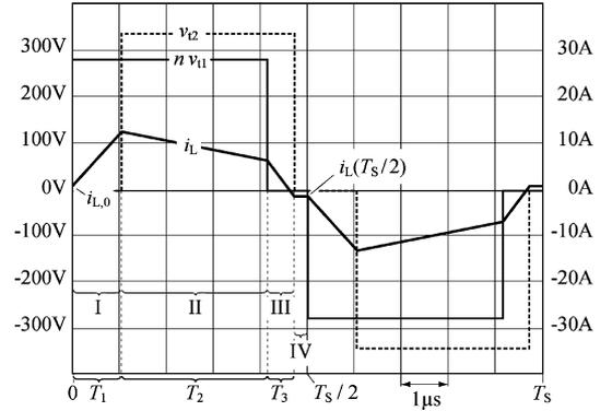
Fig. 5. Transformer voltages and inductor current for the alternative modulation and nominal operation with power transfer from the LV to the HV port ( $V_1 = 12$  V,  $V_2 = 340$  V,  $P_2 = 2$  kW). The durations of the three time intervals I, II, and III are  $T_1$ ,  $T_2$ , and  $T_3$ , respectively; the inductor current  $i_L$  is slightly negative during time interval IV in order to enable HV-side soft switching.
