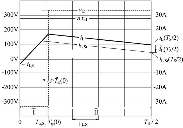
Fig. 7. Reaction of the DAB due to a phase-shift excitation  $\hat{T}_\varphi(0)$  (thick lines): at the end of the half cycle  $t = T_S/2$ , the inductor current deviation  $\hat{i}_L(T_S/2)$  results. The thin lines depict steady-state operation according to Fig. 4 (index “St” denotes “steady state”). The digital control electronics determines  $T_\varphi(0)$  at  $t = 0$ , which is applied during  $0 < t < T_S/2$ .
