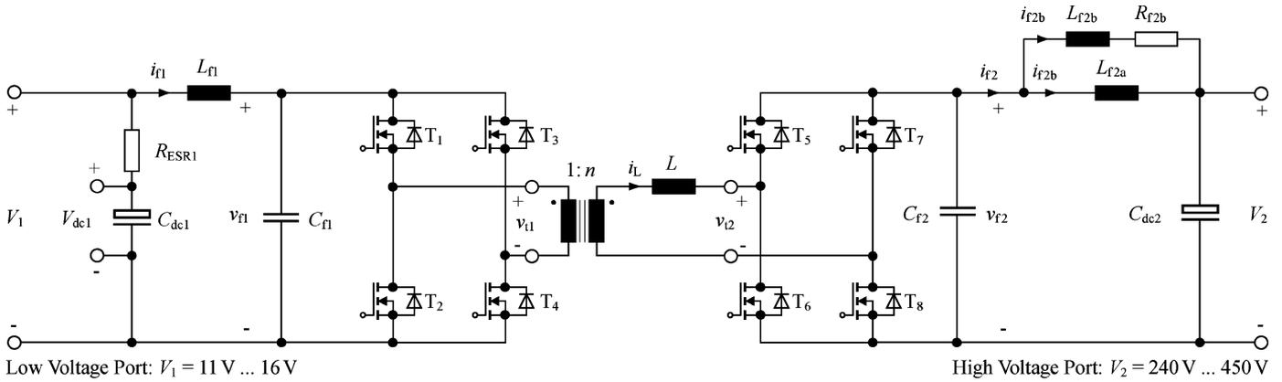
Fig. 2. DAB converter with EMI filters connected to the LV and the HV ports.
