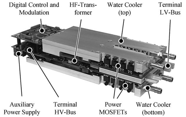
Fig. 3. Automotive DAB converter (273 mm  $\times$  90 mm  $\times$  53 mm).
