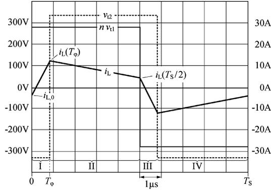
Fig. 4. Transformer voltages and inductor current for phase-shift modulation and nominal operation:  $V_1 = 12$  V,  $V_2 = 340$  V, and the HV port output power  $P_2 = 2$  kW.
