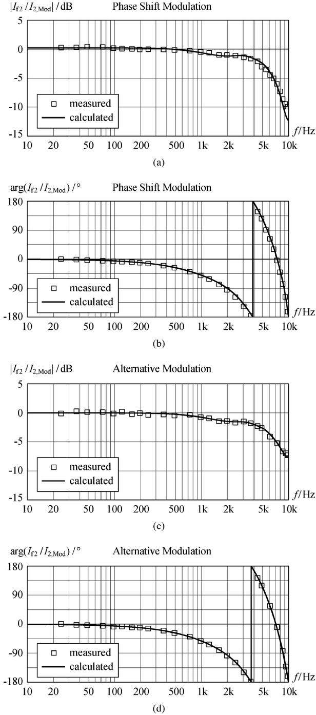
Fig. 12. Calculated and measured DAB frequency response for phase shift operation [(a) gain and (b) phase] and for the alternative modulation method [(c) gain and (d) phase]; the Nyquist frequency  $1/(2T) = 10$  kHz limits the maximum possible frequency; the solid line denotes the calculated frequency response and the boxes mark the measured values. The DAB is operated with  $V_1 = 12$  V,  $V_2 = 340$  V, and with 2 kW output power at the HV port.
