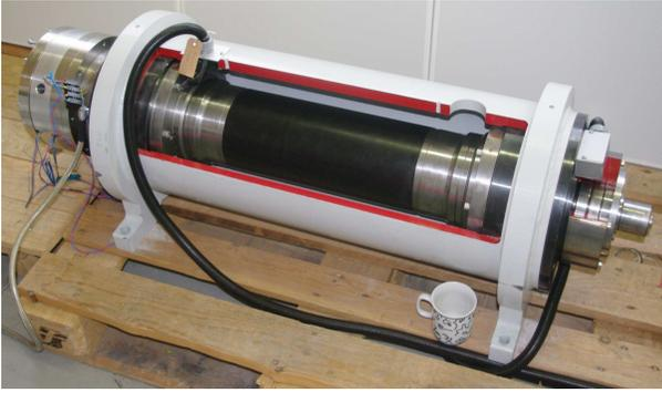
Fig. 13. Experimental bearing. The novel controller controls the attached axial bearing on the very left.
