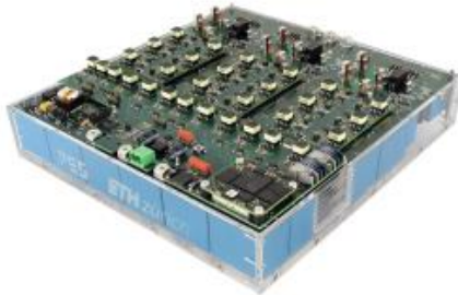
★ 7-Level All-Si HANPC PV Inverter 99.35% @ 3.4 kW/dm 3
