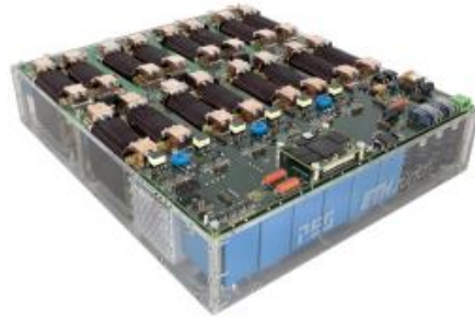
★ 3-Level All-SiC T-Type PV Inverter 99.4% @ 2.4 kW/dm 3
