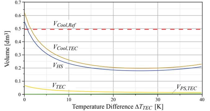
Fig. 4. Volume  $V_{Cool,TEC}$  of the cooling system with TEC and component volume as well as the volume of the conventional cooling system without TEC  $V_{Cool,Ref}$  as function of the temperature difference  $\Delta T_{TEC}$ .
