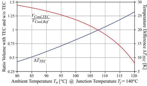
Fig. 6. Temperature difference  $\Delta T_{TEC}$  of the TEC and volume ratio between the cooling system with TEC ( $V_{Cool,TEC}$ ) and without TEC ( $V_{Cool,Ref}$ ) as function of the difference between maximal junction and ambient temperature.
