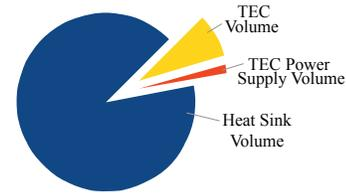
Fig. 5. Volume distribution of the cooling system with TEC for the optimal operating point  $\Delta T_{TEC}=27\text{K}$  according to Fig. 4.
