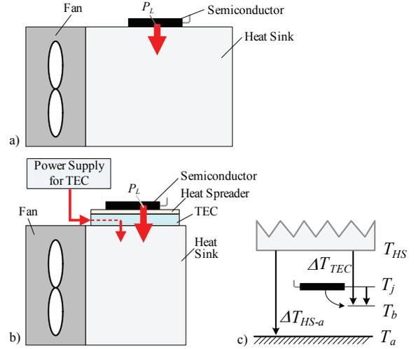
Fig. 1. a) Conventional forced air cooling system and b) high power density cooling system with thermoelectric cooler (TEC) for high ambient temperatures and limited junction temperatures. c) Temperature distribution for the cooling system with TEC. There,  $T_{HS}$  is the heat sink temperature,  $T_j$  the junction temperature,  $T_b$  the base plate temperature of the module/semiconductor housing and  $T_a$  the ambient temperature.
