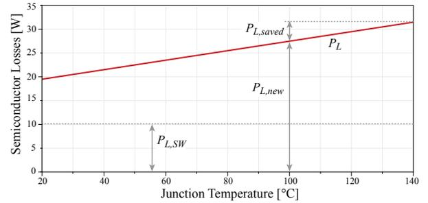
Fig. 8. MOSFET losses  $P_L$  as function of the junction temperature. By for example decreasing the junction temperature from 140°C to 100°C, losses in the amount of  $P_{L,saved}$  can be saved and only  $P_{L,new}$  must be dissipated via the heat sink and pumped by the TEC. For simplification it is assumed that the switching losses  $P_{L,SW}$  are independent of temperature.
