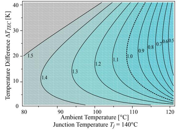
Fig. 7. Contour plot of the ratio between  $V_{Cool,TEC}$  and  $V_{Cool,Ref}$  as function of the TEC temperature difference  $\Delta T_{TEC}$  and the ambient temperature  $T_a$ . There, a fixed junction temperature of  $T_j=140^\circ\text{C}$  is assumed.
