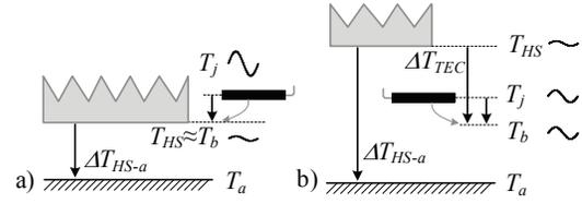
Fig. 10. a) Cooling system without TEC, where a relatively fast variation of the semiconductor losses results in a large temperature swing of the junction. b) With a TEC the temperature swing could be actively damped by distributing the amplitudes between the TEC and the junction.
