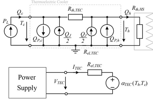
Fig. 2. Top: Electrical equivalent circuit describing the thermal behaviour of the TEC. There the heat/losses  $P_L$  injected at the cold side are transferred to the hot side, where the heat is dissipated by the heat sink. Bottom: Electric model of the TEC with auxiliary power supply.
