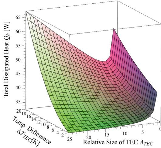
Fig. 3. Total losses  $P_{tot,HS}$ , which must be dissipated by the heat sink, for semiconductor losses of  $P_L = 31.5\text{W}$  @  $T_j = 140^\circ\text{C}$  are shown as function of the relative size of the TEC, where a size of 100% ( $A_{TEC}=1$ ) is defined by the size of the HT8-7-30, and as function of the temperature difference  $\Delta T$ . There, it is important to note, that a large size requires a large mounting area on the heat sink.
