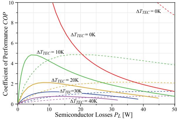
Fig. 9. Coefficient of performance  $COP$  for the TEC with the data given in Fig. 1 as function of the semiconductor losses for different temperature differences  $\Delta T_{TEC}$ . The solid line is for the original size of the HT8-7-30 and the dashed lines for a version scaled by a factor of 4 in size ( $A_{TEC} = 4$ ).
