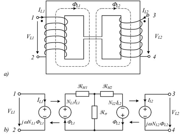
Fig. 8. Reluctance model of the integrated boost inductor of the single-phase PFC rectifier depicted in Fig. 4.
