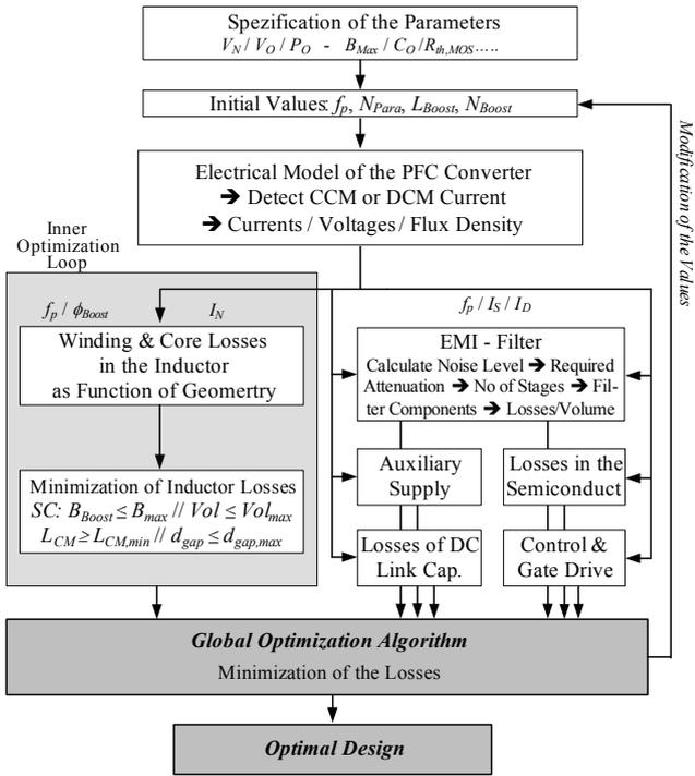
Fig. 21. Flow chart of the optimisation procedure for maximising the efficiency of the single-phase PFC rectifier shown in Fig. 4
