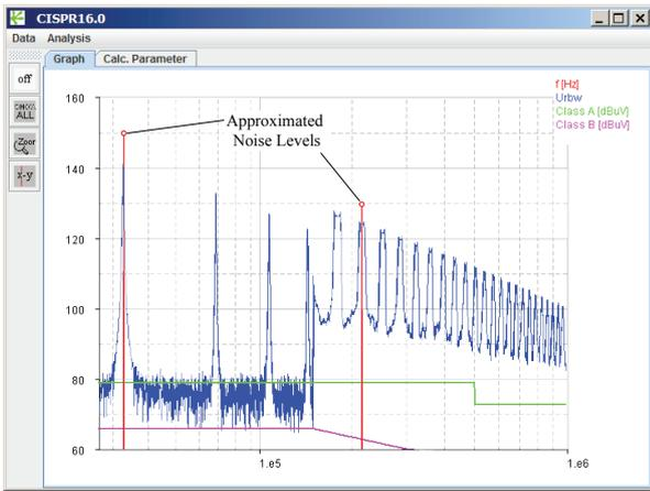
Fig. 13. Simulated noise emission of a single-phase PFC rectifier measured with an EMI test receiver in quasi-peak mode. The considered ultra-efficient PFC rectifier operates at an switching frequency of 30kHz [2], [14].
