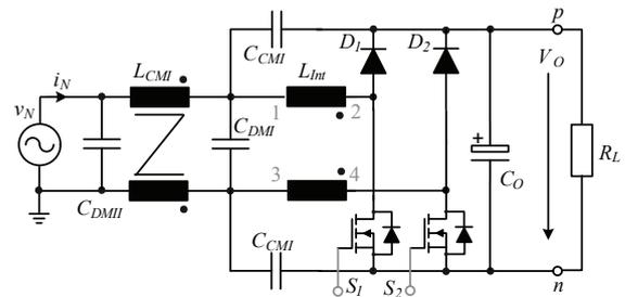
Fig. 4. Circuit schematic of the bridgeless single-phase PFC rectifier with integrated magnetics and common mode EMI filter.
