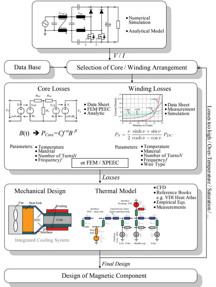
Fig. 7. Design of magnetic components applying currents and voltages determined with the electric model. With the voltages and currents the core losses and the winding losses are calculated either with analytical formulas or numerical simulations. The losses are fed into a thermal model or into a numerical simulation for determining the winding and the core temperature.
