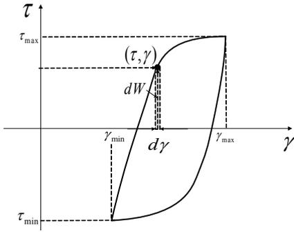
Fig. 18. Stress-strain hysteresis loop for one temperature cycle.
