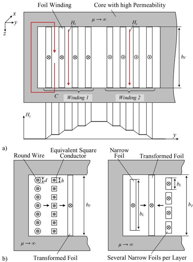
Fig. 9. a) Winding window of an E-core with two windings for a transformer. Below the E-core the distribution of the H-field is shown. b) Transformation of round wires (left) or narrow foils to an equivalent foil, which extends over the whole winding window.
