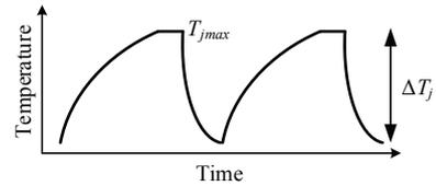
Fig. 17. A temperature cycle of a power module with peak junction temperature  $T_{jmax}$  and amplitude  $\Delta T_j$ .
