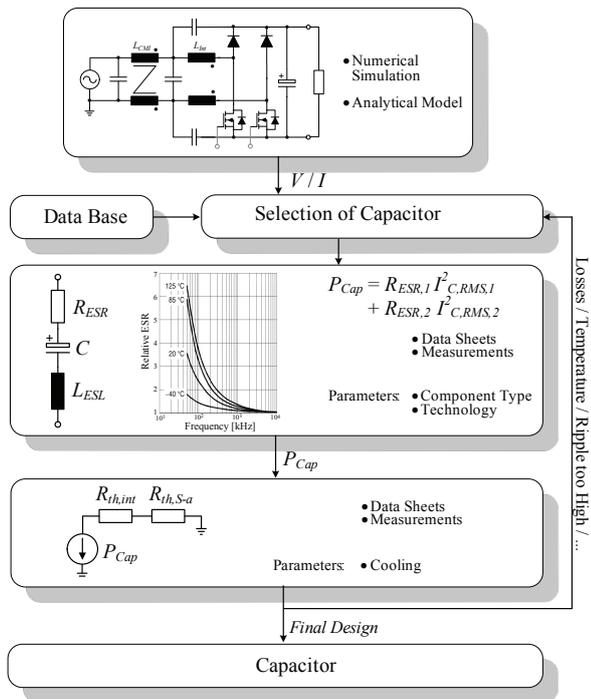
Fig. 11. Loss calculation in capacitors based on the currents/voltages resulting from the electrical model and the equivalent series resistance ESR given in the data sheet or determined by measurements. With the thermal model, which is often not given by the manufacturer, the temperature distribution within the capacitor is calculated.
