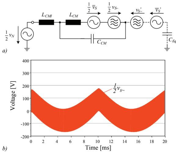
Fig. 16. CM equivalent circuit of the single-phase PFC rectifier with the parasitics given in Fig. 15. Capacitor  $C_{CM}$  represents the parallel connection of the two capacitors  $C_{CMI}$ , i.e.  $C_{CM} = 2C_{CMI}$ . With a varying potential of the negative DC output rail  $n$ , also a CM current is flowing via capacitors  $C_S$ ,  $C_p$  and  $C_n$ . There, additionally the CM voltage  $v'_S$  must be considered.
