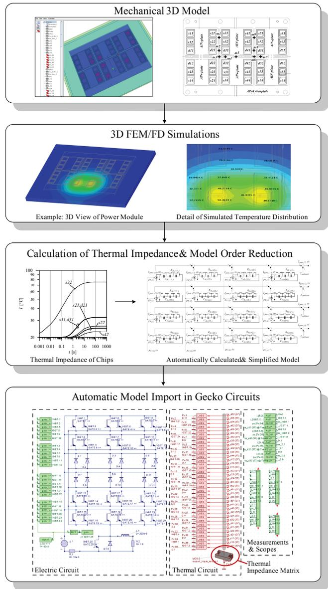
Fig. 23. Flowchart of an automatic generation of a thermal equivalent circuit based on a 3D mechanical design, FEM simulations and an automatic model order reduction. Finally, the equivalent circuit of the power module or of different semiconductors on a heat sink is directly imported into GeckoCIRCUITS<sup>TM</sup> and could be used to calculate the junction temperatures.
