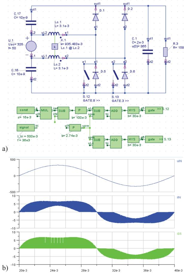
Fig. 5. a) Electrical simulation of the single-phase PFC rectifier given in Fig. 4 without EMI filter implemented in GeckoCIRCUITS<sup>TM</sup> [12]. b) Simulated mains voltage, mains current, and transistor current.
