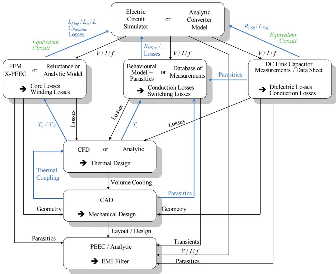
Fig. 22. Models for the different domains with the data exchange shown by black arrows. Examples for coupling of different domains are shown by blue arrows.
