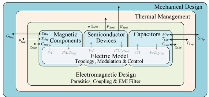
Fig. 24. Diagram showing the inter-domain couplings. These couplings are arranged such, that the domains which influence other domains are enclosing these domains. There, the main direction of influence is considered and e.g. the influence of the parasitics on the losses, i.e. the design of the cooling system, is neglected.
