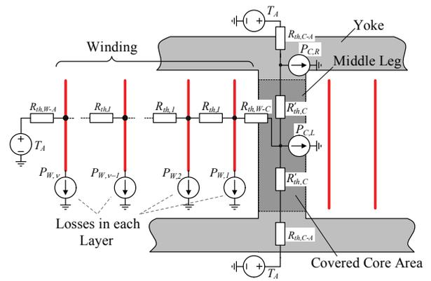
Fig. 10. Thermal model for a magnetic device with an E-core and foil windings. The insulation between the layers is represented by a thermal resistance and each turn generates its own losses. Also the core is split into different sections. There, especially the middle leg, around which the foil winding is wound, is important, since there also losses from the winding are transferred to the core.
