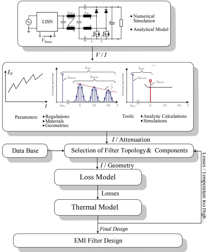
Fig. 12. Design of the DM EMI filter based on simulated input currents and the calculated LISN output voltage. Based on an approximative routine, which determines the required attenuation based on the noise emission level and the limits, the values of the filter inductance and capacitance are calculated. There, the input current as well as the LISN output voltage could also be calculated analytically.
