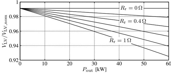
Fig. 4. Dependence of the LV side output voltage on the transferred power and the resistor  $R_r$ .
