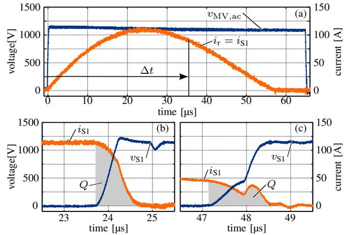
Fig. 8. (a) Positive current pulse where the current through  $S_1$  equals the current  $i_r$  for  $L_\sigma = 7.6$   $\mu$ H and  $C_r = 43$   $\mu$ F, resulting in  $f_0 \approx 8.8$  kHz. The turn-off time is defined by  $\Delta t$  and varied to measure the extracted charge at different points of the current waveform. Definition of the charge extracted from  $S_1$  for (b)  $\Delta t = 24$   $\mu$ s and (c)  $\Delta t = 48$   $\mu$ s.
