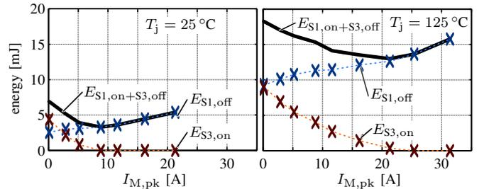
Fig. 12. Influence of the magnetizing current peak value,  $I_{M,\text{pk}}$ , on the turn-off losses in  $S_1$  and the turn-on losses in the complementary switch  $S_3$ .
