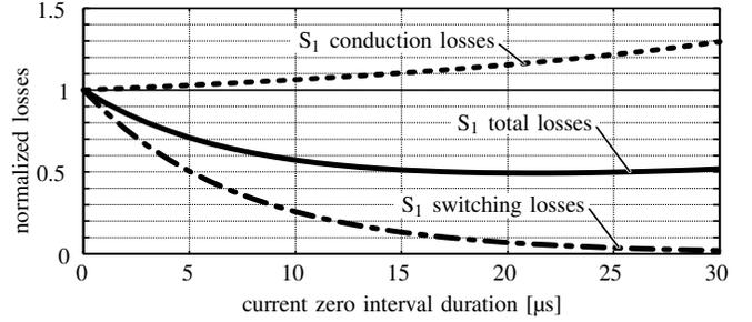
Fig. 10. Influence of the zero current interval duration on the semiconductor losses for  $f_s = 7.5\text{ kHz}$  and  $T_j = 125\text{ }^\circ\text{C}$ . Note that the optimum is shifted to the left and upwards if other losses related to rms current are included.
