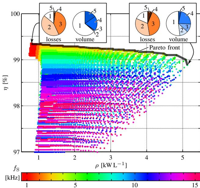
Fig. 16. Resulting designs in the  $\eta\rho$ -plane with  $C_P = 0.7$ ; the Pareto front is highlighted and relative loss and volume distribution for the two extreme points of the Pareto front are shown: 1) transformer, 2) LV semiconductors, 3) MV semiconductors, 4) DC links, 5) resonant capacitors.
