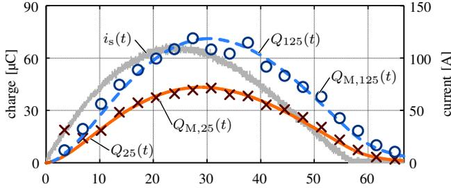
Fig. 9. Behavior of the stored charge for the FF150R17KE4 IGBT at  $T_j = 25\text{ }^\circ\text{C}$  and  $T_j = 125\text{ }^\circ\text{C}$ .  $Q_{M,25}(t)$ ,  $Q_{M,125}(t)$  are measurements and  $Q_{25}(t)$ ,  $Q_{125}(t)$  are obtained with (14) and  $k_s$ ,  $\tau$  as given in Table II.
