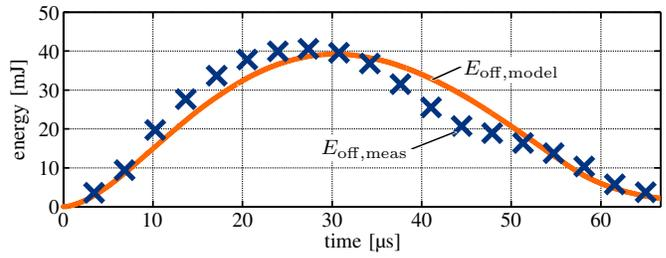
Fig. 14. Measurement and estimate of the turn-off losses in  $S_1$  at  $T_j = 125$  °C. The  $\Delta t$  values used for the measurements are the same as in Fig. 9.
