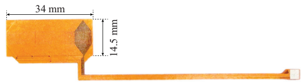
Fig. 2. Photograph of the radial position sensor before being rolled and inserted in the stator bore. The sensor is realized as a two-layer flexible printed circuit. Copper thickness is 35 \mu\text{m} and the diameter of via holes is 0.1 mm.
