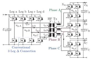
**Fig. 1:** Proposed multi-port DC/DC converter topology formed by integrating the primary converter stages of three dual active bridge converters (DABCs) into a four-leg inverter. The resulting topology is named 4L3 QABC, indicating three controllable DC outputs operated by three independent DABCs, abbreviated as phases A, B, and C. The dotted line denotes the known three-leg inverter topology (3L3 QABC), as referenced in [12], [13].
