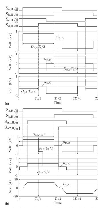
**Fig. 2:** Typical operation waveforms of the 4L3 QABC when all duty cycles are set as  $D_{\{\mathrm{p,s}\},\{\mathrm{A,B,C}\}}=0.8$ , and phase shifts are set as  $\phi_{\{\mathrm{A,B,C}\}}=\pi/9$ : (a) Gate signals of the high-side of the four-leg inverter and its output voltages to the primary side terminals of the HF transformers. (b) Gate signals, imposed voltages to the primary and secondary side terminals of the HF transformers, and the transformer current of phase A of the 4L3 QABC.
