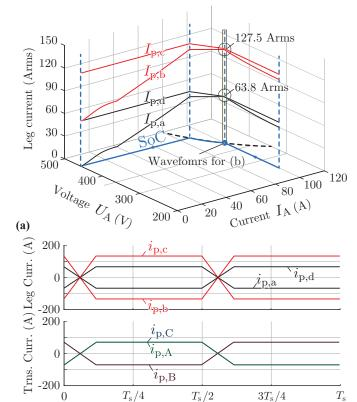
**Fig. 4:** Four-leg inverter leg current characteristics under *Case 1*: (a) Current RMS value of the leg current across the SoC. (b) Leg currents  $i_{\rm p,\{a,b,c\}}$  and transformer currents  $i_{\rm p,\{A,B,C\}}$  on the primary side at the rated operation for all phases.
