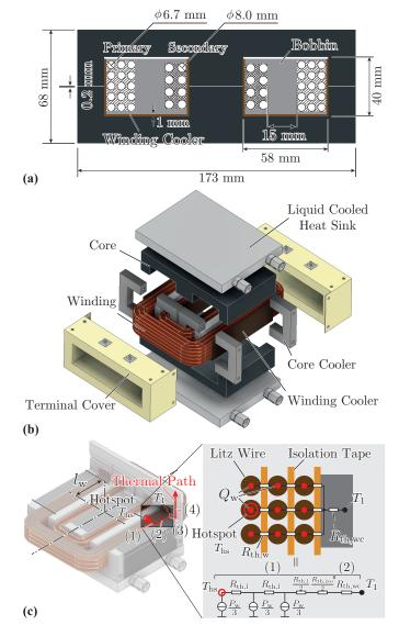
**Fig. 6:** Designed single-phase transformer featuring a total power of  $40\,\mathrm{kW}$ , an efficiency of  $99.68\,\%$  with  $31.9\,\mathrm{W}$  core loss, and  $94.5\,\mathrm{W}$  winding loss: (a) Geometric parameters of the transformer, yielding  $17.7\,\mu\mathrm{H}$  leakage inductance. (b) Cooling system assembly with winding and core cooler, referred to in [29]. (c) The hotspot in the winding and its thermal path to the heat sink in an evenly octant-divided transformer.
