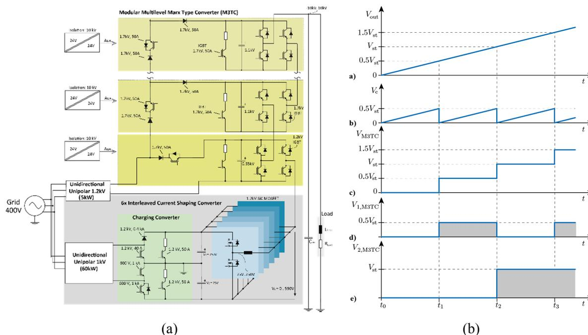
Fig. 4: (a) Stack module of the current source, with 1.5kA nominal current and  $\pm 10$ kV output voltage per stack. The full-scale source consists of 20 parallel stacks with a nominal current of 30kA. (b) Basic operating principle of the investigated current source. a) Output voltage  $V_{out}$ . b) Converter output voltage  $V_c$ . c) M3TC voltage  $V_{M3TC}$ . d) Voltage of the first stage of the M3TC. e) Voltage of the second stage of the M3TC [25].
