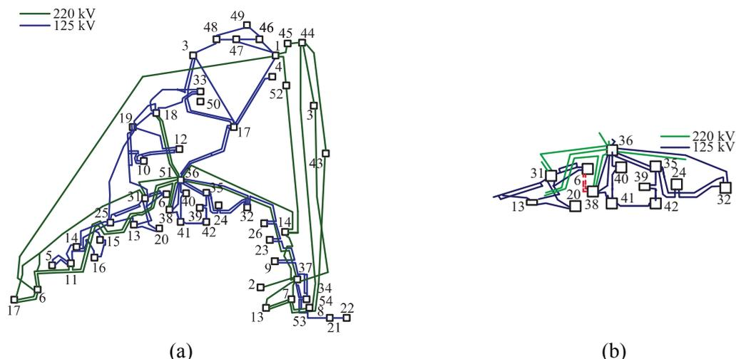
Fig. 5: (a) Single line diagram of transmission and distribution networks of the Geneva region. (source: Romande Energie). (b) New line location.
