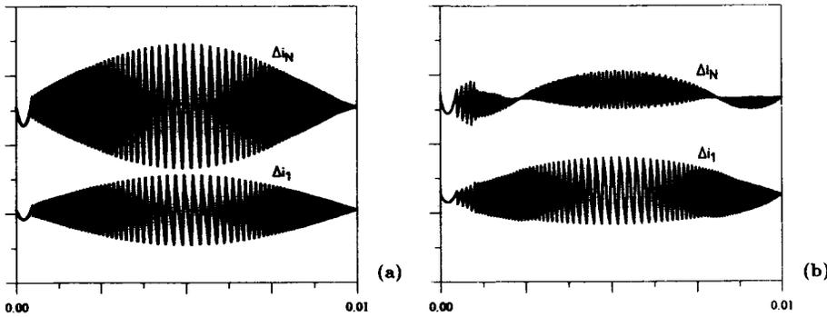
Fig.8: Time shapes (corresponding to Fig.7) of the ripple  $\Delta i_1$  of the partial current  $i_1$  and of the ripple  $\Delta i_N$  of the total current  $i_N$ . (a):  $T_i = 0$  (cf. Fig.7(a) and (b)); (b):  $T_i = 6.5 \mu s$  (cf. Fig.7(c) and (d)); scales: 2.5 ms/div, 2.5 A/div.
