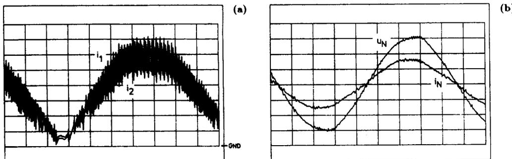
Fig.9: Experimental analysis of the self-adjusting staggered switching of an AC-DC boost power factor corrector according to Fig.2. (a): input currents  $i_1$  and  $i_2$  of the partial systems (0.5 A/div); (b): total input current  $i_N$  of the system (4 A/div) and mains voltage  $u_N$  (50 V/div). Time scale: for (a): 1 ms/div, for (b): 2 ms/div.
