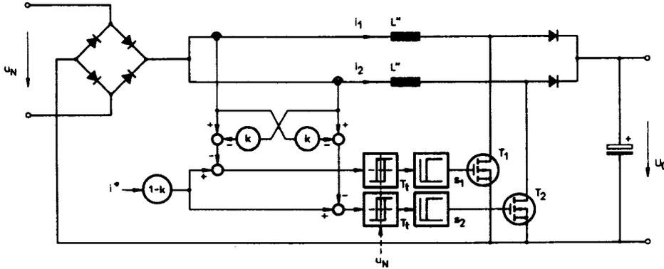
Fig.10: Structure of the circuit according to Fig.2 if the inductance  $L_N$  (coupling the partial systems) is replaced by a coupling  $k$  of the current control loops. The apparent reduction (due to the coupling) of the partial currents has to be considered by a factor  $(1 - k)$  in the reference value path of the current control.
