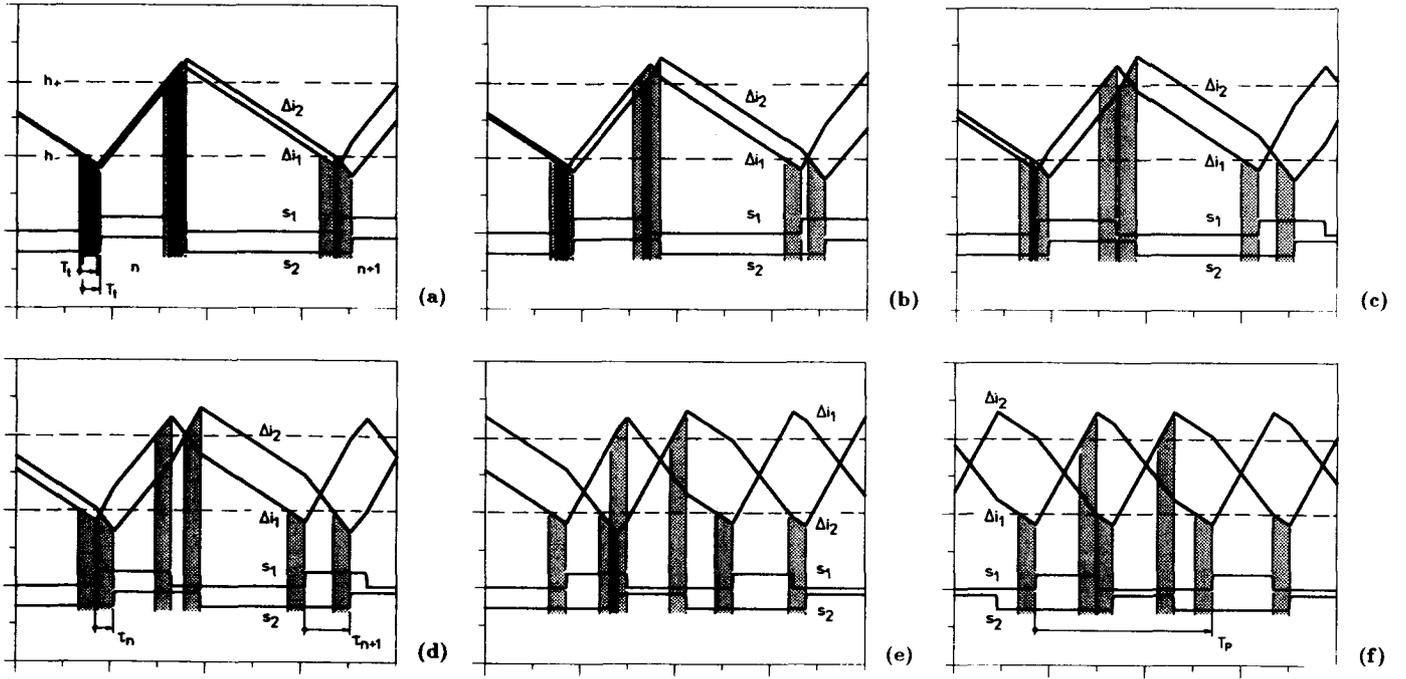
Fig.5: Representation of the shapes of the current ripples  $\Delta i_1$  and  $\Delta i_2$  and switching functions  $s_1$  and  $s_2$  as being characteristic for the cases A - F to be distinguished for the mathematical analysis of the locking process. The denomination of the figures corresponds to the related calculation region. E.g., (a) corresponds to region A, (f) corresponds to the region of stationary operation F.
