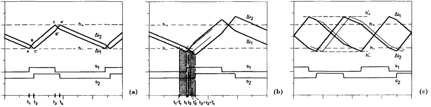
Fig.4: Shape of the current ripples  $\Delta i_1$  and  $\Delta i_2$  and of the switching functions  $s_1$  and  $s_2$  of the circuit according to Fig.2 for  $T_i = 0$  (cf. (a)) and  $T_i = 6.5 \mu s$  (cf. (b) and (c)); the remaining simulation parameters are equal as for Fig.1(b) or Fig.3(c); time scale:  $27.5 \mu s/\text{div}$ .
