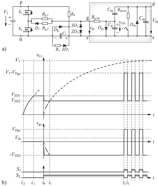
**Fig. 5:** a) Moving the described gate drive circuitry from the gate to the source connection and swapping the polarity of  $D_k$ ,  $ZD_1$  enables a simple charging of  $C_s$  through  $R_4$  before the first turn-on sequence at  $t_2$  is taking place and b) corresponding waveforms during start up.
