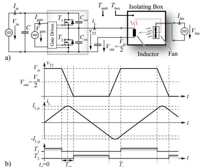
**Fig. 8: a)** Calorimetric measurement setup used to determine the soft-switching losses and **b)** waveforms of the bridge voltage  $v_{T2}$ , the inductor current  $i_L$  and the appropriate gate signals of the two switches  $T_1$  and  $T_2$ .
