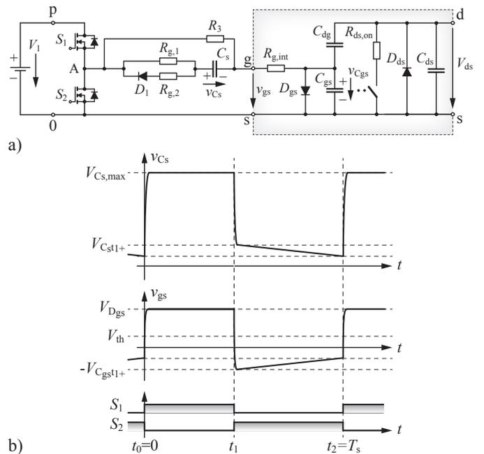
**Fig. 3:** a) GaN gate drive circuit with decoupling capacitor  $C_s$  as proposed in [11] and b) corresponding waveforms during one switching cycle.
