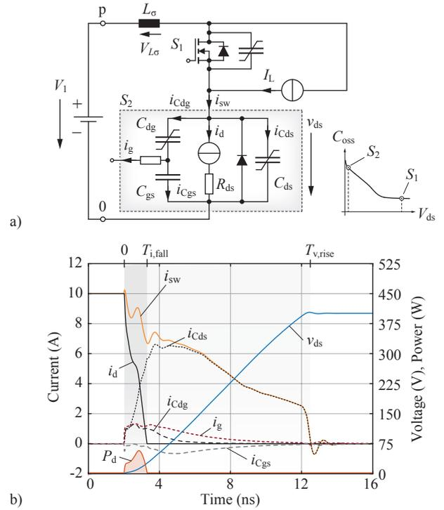
**Fig. 6:** Analysis of the soft-switching turn-off transition with **a)** the capacitive model of the MOSFET and **b)** the turn-off transition simulated with Gecko Circuits considering the non-linear MOSFET capacitances and parasitic inductances.
