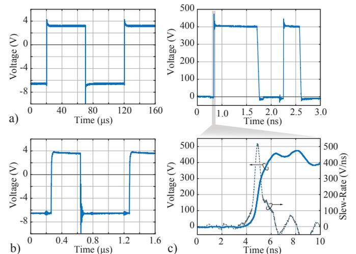
**Fig. 7:** Measured gate voltages for the two switching frequencies **a**)  $f_{\text{s}} = 10 \text{ kHz}$  and **b**)  $f_{\text{s}} = 1 \text{ MHz}$  and **c**) the measured maximum voltage slope of above  $500 \text{ kV}/\mu\text{s}$  achieved with hard switching.
