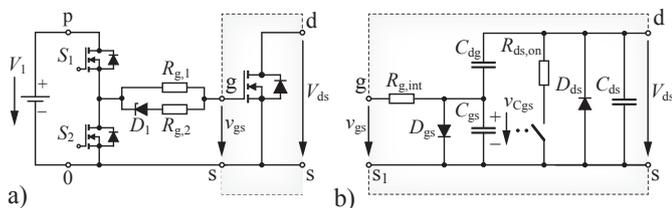
**Fig. 2:** a) Conventional gate drive circuit for voltage controlled semiconductor devices with separate gate resistance for on- and off-transition and b) simplified equivalent circuit of the GaN GIT describing the gate input behavior.
