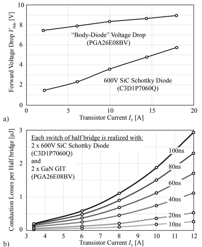
**Fig. 11:** Measured conduction losses due to the additional conduction of the anti-parallel diode during the commutation interval.
