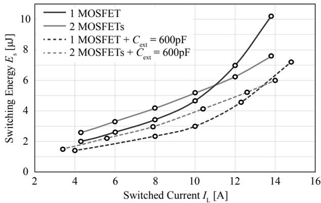
**Fig. 10:** Measured soft-switching losses  $E_s$  depending on the switched current  $I_s$  for four different half-bridge assemblies.
