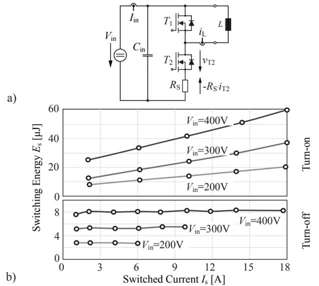
**Fig. 9: a)** Double pulse test setup used to perform the hard-switching loss measurements and **b)** measured hard-switching losses  $E_s$  (turn-on and turn-off) depending on the switched current  $I_L$  and the input voltage  $V_{in}$ .
