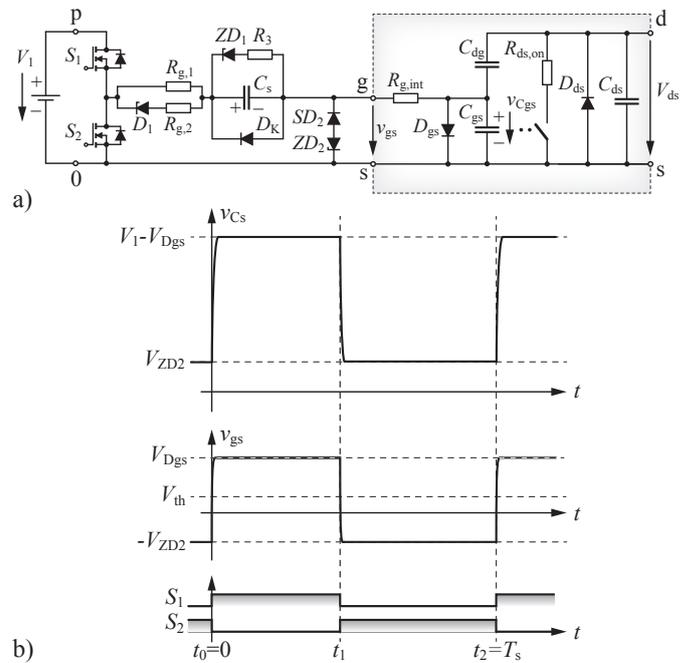
**Fig. 4:** a) Improved GaN gate drive circuit showing the proposed modification in the gate drive's driving part in order to guarantee a safe gate drive operation with consistent performance and b) corresponding waveforms during on switching cycle.
