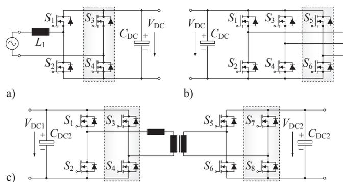
**Fig. 1:** Typical bridge leg applications: **a)** Totem-pole PFC full-bridge rectifier, **b)** Totem-pole full-bridge inverter, **c)** DC-DC dual active bridge.
