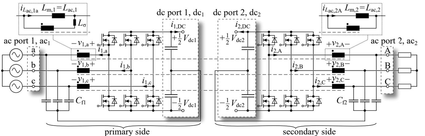
**Fig. 1.** Dual Three-Phase Active Bridge (D3AB) topology with a ac and dc port on primary side ( $ac_1$ ,  $dc_1$ ) and a galvanically isolated ac and dc port ( $ac_2$ ,  $dc_2$ ) on the secondary side.
