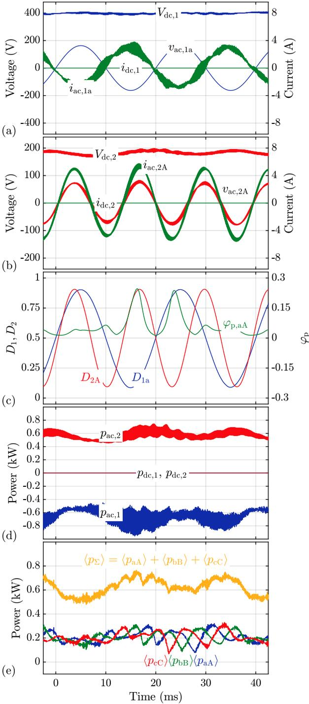
**Fig. 9.** Circuit simulation results for  $ac_1$ – $ac_2$  operation with  $V_{dc,1} = 400$  V,  $V_{dc,2} = 200$  V,  $V_{ac1,rms} = 115$  V,  $V_{ac2,rms} = 57.5$  V,  $f_1 = 50$  Hz,  $f_2 = 77$  Hz, and a resistive load with  $R_{load} = 14.7 \Omega$  on each phase of  $ac_2$  resulting into  $p_{ac,2} = 675$  W.
