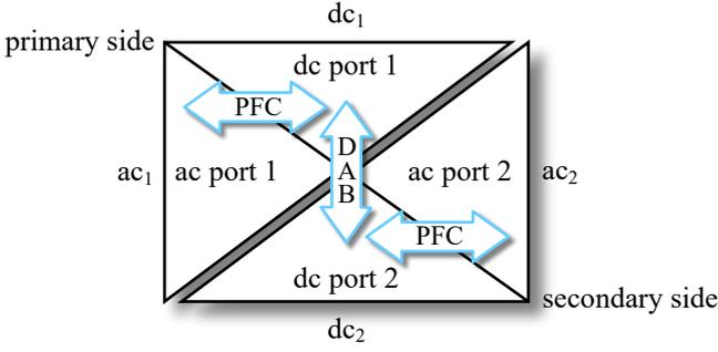
**Fig. 4.** The power transfer between the four ports of the D3AB converter can be separated into  $ac_1$ – $dc_1$  and  $ac_2$ – $dc_2$  operation w/o galvanic isolation and  $dc_1$ – $dc_2$  operation w/ galvanic isolation. For  $ac_1$ – $dc_1$  and  $ac_2$ – $dc_2$  the corresponding VSCs is operated according to (7) and (8) to achieve Power Factor Correction (PFC) functionality. The power transfer  $dc_1$ – $dc_2$  is utilizing the DAB functionality.
