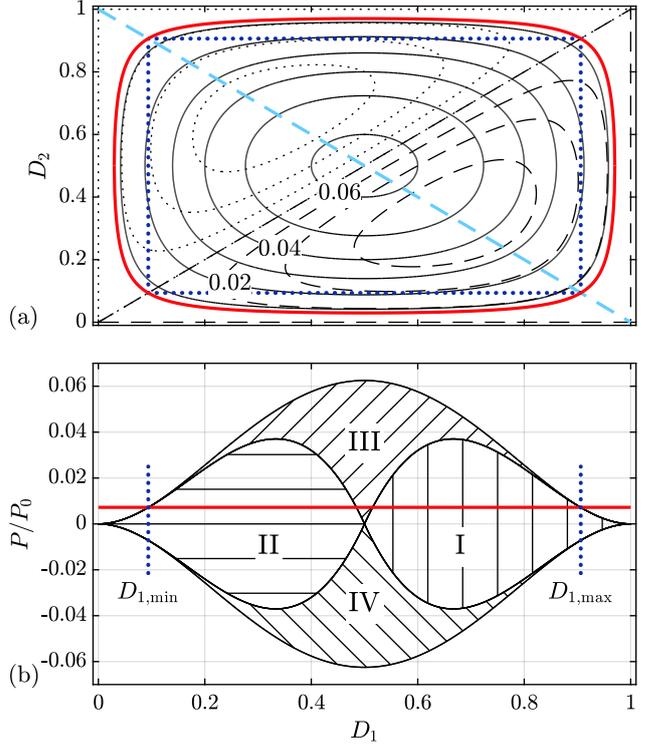
**Fig. 7.** (a) Contour plot of the maximum power for modes I to III and (b) cut along the dashed light-blue line through the maximum power contour plot. Red line represents a solution with constant power in each phase.
