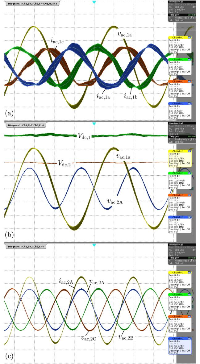
**Fig. 10.** Measurement results with same conditions as for the circuit simulation Fig. 9. (a) Sinusoidal currents at  $ac_1$  [2 A/div] and the phase voltage of phase a [50 V/div] as a reference; (b) both dc-link voltages [100 V/div] and phase a voltages [50 V/div] of primary and secondary side; (c) sinusoidal voltages at  $ac_2$  [50 V/div] and the current of phase a [2 A/div] as a reference. All measurements are synchronized and have a time resolution of [5 ms/div].
