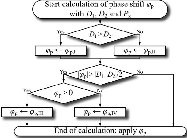
**Fig. 6.** Algorithm used to identify the current mode each DAB converter phase is operated in and to calculate the corresponding phase shift  $\varphi_p$ .
