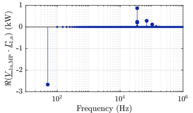
**Fig. 3.** Power transferred in a single phase, e.g., phase a, in frequency domain for the  $ac_1$ – $dc_2$  operation described in [7] with line frequencies  $f_m = 50 \text{ Hz}$  and a switching frequency of  $f_s = 35 \text{ kHz}$ .
