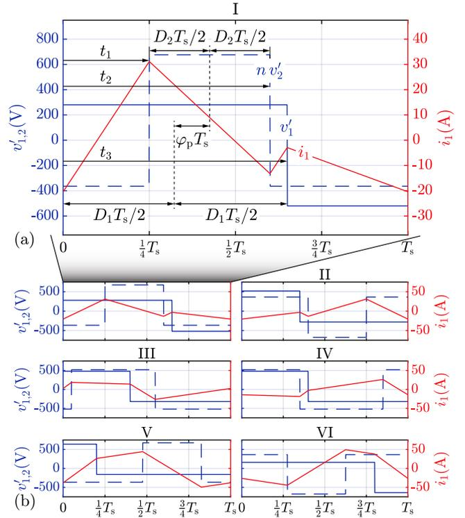
**Fig. 5.** (a) Definitions of  $D_1$ ,  $D_2$ , and load angle  $\varphi$  with calculated waveforms over one switching period,  $T_s$ , with  $f_s L_\sigma \approx 3.4 \Omega$ ,  $n = 2.6$ ,  $V_{dc1} = 800 \text{ V}$ ,  $V_{dc2} = 400 \text{ V}$ ,  $D_1 = 0.4$ ,  $D_2 = 0.5$  and  $\varphi \approx 29^\circ$  and (b) all possible operation modes for this DAB converter.
