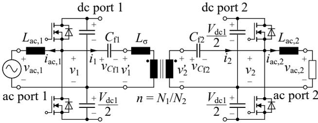
**Fig. 2.** Single-phase equivalent system with the two boost inductances  $L_{ac,1}$  and  $L_{ac,2}$ , the stray inductance  $L_{\sigma}$ , and the isolating HF transformer with turns ratio  $n$ .
