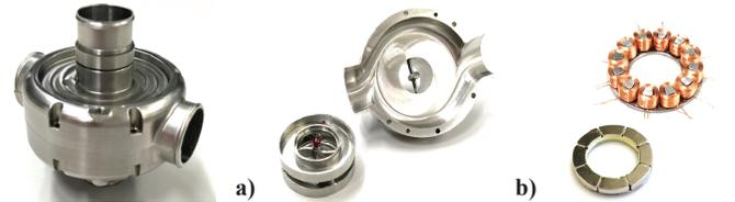
Fig. 10. Pump prototype parts: a) titanium housing and impeller of the implantable blood pump and b) stator and PM rotor of the motor prototype with a pole-pair number of  $p = 4$  and a stator height of  $h_s = 3.8$ .
