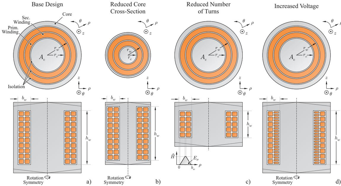
Figure 4: Scaling of the MF transformer for changes in operating frequency and voltage (drawings are not to scale): a) Base design; b) Adaptation of the core cross section  $A_c$  to account for operating frequency  $f_s$  increase; c) Modification of a) in the number of turns  $N_1$  to account for operating frequency  $f_s$  increase; d) Increase of number of turns  $N_1$  to enable operation with higher voltages.
