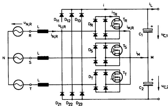
Fig.2: Basic structure of a three-phase/switch/level unity power factor PWM rectifier resulting by further development of of Fig.1(d); the feeding mains is replaced by a voltage sources  $u_{N,i}$ ,  $i = R, S, T$ .
