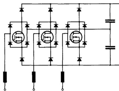
Fig.9 Structure of the power circuit of a three-phase/switch/level PWM rectifier when the control elements  $T_i$  and  $D_i$ ,  $i = R, S, T$ , are integrated into the associated legs of the three-phase diode bridge on the input side (cf. Fig.2).
