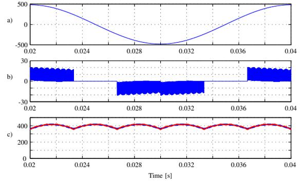
Fig. 3. Performance of the GPU in the dc-side without the input filter and the injection circuit: a) power source voltage  $v_{sA}[\text{V}]$ ; b) ac line current  $i_{sA}[\text{A}]$ ; c) capacitor voltages  $v_{dc1}[\text{V}]$  (red line),  $v_{dc2}[\text{V}]$  (blue line).
