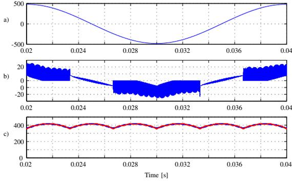
Fig. 5. GPU performance with the active current injection: a) source voltage  $v_{sA}$  [V]; b) source current  $i_{sA}$  [A]; c) capacitor voltages  $v_{dc1}$  [V] (red line),  $v_{dc2}$  [V] (blue line).
