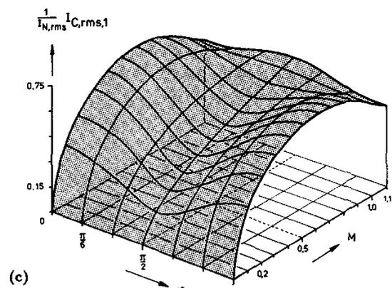
**Fig.5:** Dependency of the inverter-side contribution  $I_{C,\text{rms},1}$  (cf. Eq.(27)) to the global DC link capacitor current rms value  $I_{C,\text{rms}}$  on the inverter modulation index  $M$  and on the phase displacement  $\varphi$  of the fundamentals of the inverter output phase voltages  $u_{U,i}$  and the associated output phase currents  $i_{N,i}$ . Parameters of the family of curves:  $\cos \varphi$  (cf. (a)) and  $M$  (cf. (b)); (c): three-dimensional representation.
