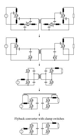
Fig. 8. Systematic synthesis of the flyback converter (step 5): Simplification of the circuit obtained in Fig. 7 results in the circuit of a flyback converter with clamp switches. Note that the two inductors of the final circuit are magnetically coupled.
