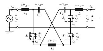
Fig. 10. Final simplified circuit obtained from the synthesis of a novel nonisolated single-phase buck-boost AC-DC converter in Fig. 9.
