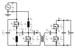
Fig. 14. Simplified circuit of the isolated single-phase PFC rectifier in Fig. 13.
