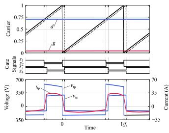
Fig. 17. Simulated gate signals and transformer waveforms (at 20 ms) of the isolated single-phase PFC rectifier in Fig. 14.
