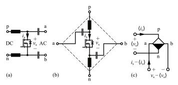
Fig. 2. Elementary converter. (a) Circuit structure and (b) re-arrangement leading to (c) schematic symbol of the elementary converter with DC terminals p, n, and AC terminals a, b.
