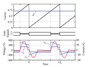
Fig. 18. Simulated gate signals and transformer waveforms of the isolated rectifier in Fig. 14 with diodes instead of MOSFETs on the secondary side and series compensated transformer leakage inductance.
