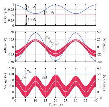
Fig. 11. Simulated input/output waveforms of the non-isolated single-phase buck-boost PFC rectifier in Fig. 10.
