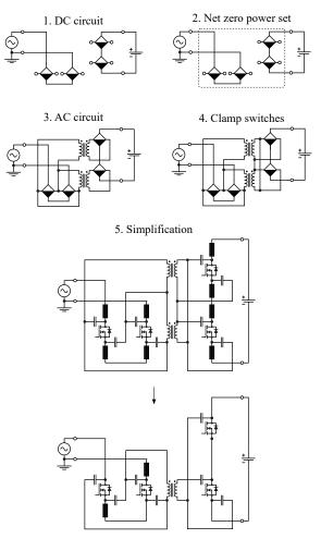
Fig. 13. Synthesis of an isolated single-phase PFC rectifier.
