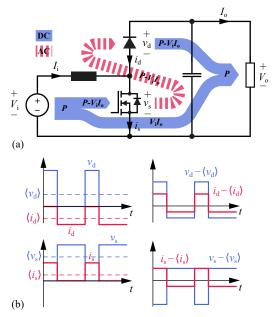
Fig. 1. (a) Boost converter circuit and power flows and (b) idealized switch and diode voltage and current waveforms separated into their DC and AC components.
