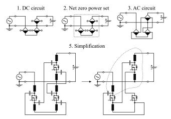
Fig. 9. Synthesis of a novel non-isolated single-phase buck-boost AC-DC converter. One of the three encircled inductors is redundant and can be shorted, leading to three different circuit variants; one is shown in Fig. 10.
