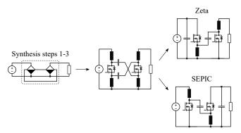
Fig. 6. Synthesis of a non-inverting buck-boost converter results in either the Zeta converter or the SEPIC converter, depending on which of the redundant inductors are removed.
