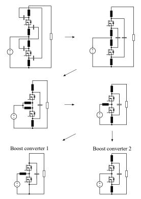
Fig. 4. Systematic synthesis of the boost converter (step 5): Simplification of the converter circuit obtained in Fig. 3; note that in the last step two different final results with identical terminal behavior can be achieved by shorting either one or two of the inductors.
