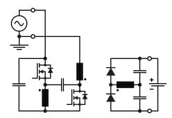
Fig. 19. Unidirectional circuit variant of the isolated single-phase PFC rectifier from Fig. 14 with integrated transformer; note that all inductors are magnetically coupled.
