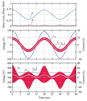
Fig. 16. Simulated input/output waveforms of the isolated single-phase PFC rectifier in Fig. 14.
