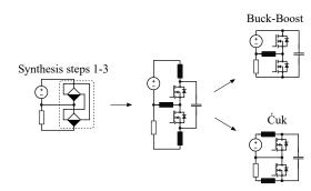
Fig. 5. Synthesis of an inverting buck-boost converter results in either the buckboost converter or the Ćuk converter, depending on which of the redundant inductors are removed.
