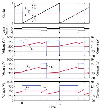
Fig. 12. Simulated switch waveforms (at 7 ms into the mains period) of the non-isolated single-phase buck-boost PFC rectifier in Fig. 10.
